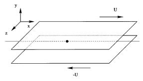
FIG. 1. Modified Couette flow apparatus.
