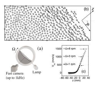
FIG. 1. (a) Sketch of the experimental setup. (b) A typical instanteous velocity field obtained for quasi-2D flows (geometry A) with  $\Omega = 8$  rpm in the rectangular box of (a). (c) Velocity profile measured at the center of the drum for three different rotation speeds:  $\Omega = 1$  rpm,  $\Omega = 3$  rpm, and  $\Omega = 8$  rpm. The arrows indicate the end of each profile. The precision on each point is better than the point size.
