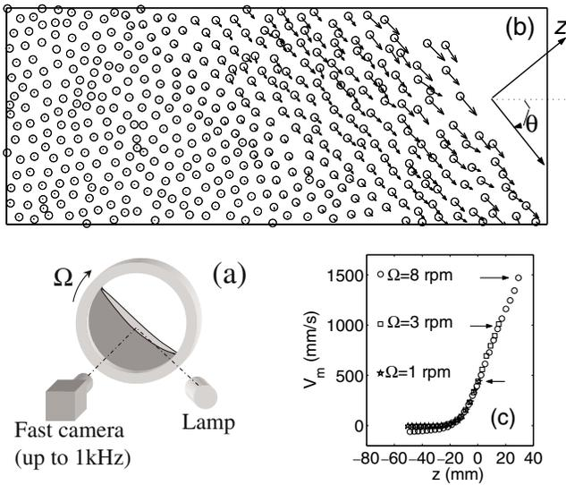
FIG. 1. (a) Sketch of the experimental setup. (b) A typical instantaneous velocity field obtained for quasi-2D flows (geometry A) with  $\Omega = 8$  rpm in the rectangular box of (a). (c) Velocity profile measured at the center of the drum for three different rotation speeds:  $\Omega = 1$  rpm,  $\Omega = 3$  rpm, and  $\Omega = 8$  rpm. The arrows indicate the end of each profile. The precision on each point is better than the point size.
