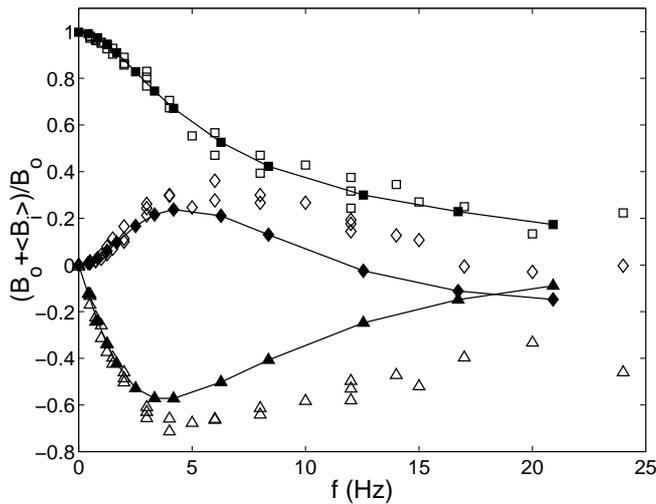
**Fig. 15.** Comparison with the VKS experiment in the case of one rotating TM60 disk. Diamonds, squares and triangles respectively refer to  $B_x$ ,  $B_y$  and  $B_z$ . The dark symbols and solid lines correspond to the predicted response to a uniform transverse magnetic field based on the velocity field used in the experiment. The white symbols correspond to the measured data.
