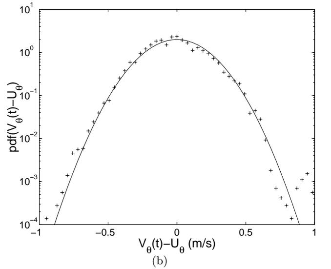
**Fig. 2.** (a) Temporal evolution of the fluctuating part of the azimuthal velocity of TM60 propeller recorded using Laser Doppler Velocimetry at  $r = 60$  mm,  $z = 65$  mm for  $f = 2$  Hz. The value of the mean azimuthal velocity is  $U_\theta = 0.42$  ms $^{-1}$ . (b) Probability density function for the same signal: data (+) and Gaussian fit (solid line).
