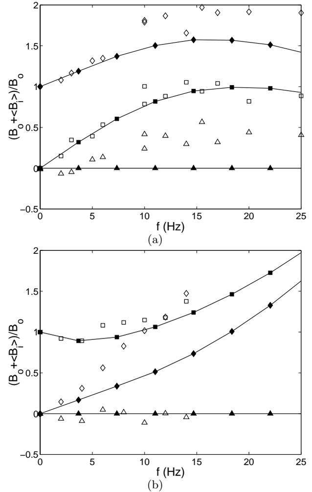
**Fig. 14.** Comparison with the VKS experiment in the case of 2 counter-rotating TM60 propellers. Response to an axial (a) and a uniform transverse (b) magnetic field. Diamonds, squares and triangles respectively refer to  $B_x$ ,  $B_y$  and  $B_z$ . The dark symbols and solid lines correspond to the predicted behavior based on the velocity field used in the experiment. The white symbols correspond to the measured data.
