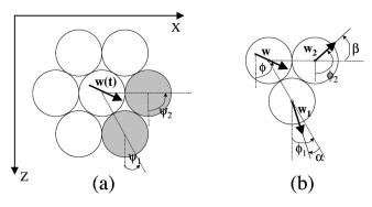
FIG. 3. Propagation rule of the overload from a given bead to two of its neighbors. (a) The orientation  $\phi$  of the load  $\mathbf{w}$  determines the two neighbors  $P_1$  and  $P_2$  which will support this charge. (b) The orientations  $\phi_1$  and  $\phi_2$  of the two *children* charges resulting from the transmission coincide with the two contact orientations  $\psi_1$  and  $\psi_2$  at which two random numbers  $\alpha$  and  $\beta$  have been added, respectively.
