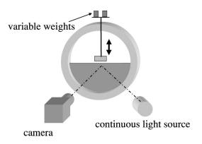
FIG. 1. Sketch of the experimental setup.
