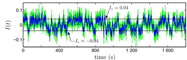
FIG. 3 (color online). Global angular momentum  $I(t)$  as a function of time for an experiment performed at  $\text{Re} = 43\,000$  for  $\theta = 0$ . Green (light gray) dots are PIV data sampled at 15 Hz, and blue (dark gray) dots correspond to 1 Hz low-pass filtered data  $I_f(t)$ . Eye-guiding lines have been drawn at  $I(t) = \pm I_* = \pm 0.04$ .
