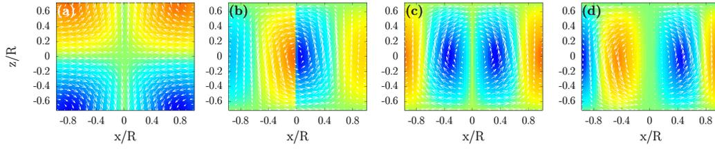
FIG. 2. (a) (resp., (b), (c), and (d)) synthetic velocity field  $\mathbf{b}^{\text{nmk}}$  obtained from corresponding Beltrami modes  $\mathbf{B}^{\text{nmk}}$  in a meridional plane with  $n = k/k_0 = 1$  and  $m = 0$  (resp.,  $m = 1, 2$ , and  $3$ ). Same color and arrow codes as in Fig. 1.
