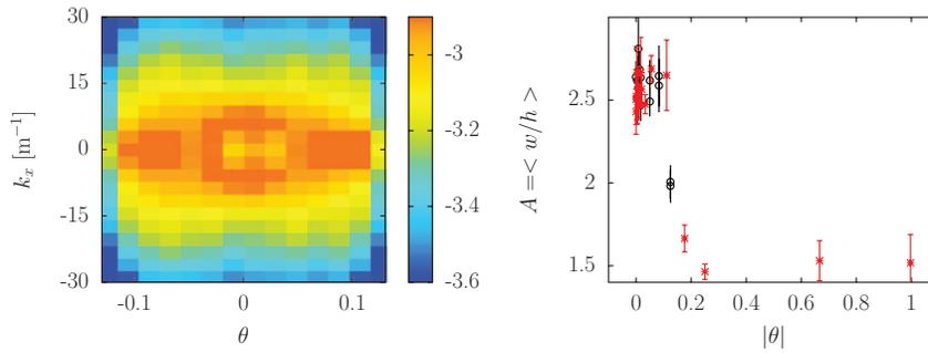
FIG. 7. Left, experimental spatio-temporal spectrum  $E_E(k_x, \theta)$  at  $\text{Re} \approx 10^5$ . The shear layer reaches the slower impeller at  $\theta = \pm 0.1$ . Colors are log scaled. Right,  $A = \langle w/h \rangle$  as defined in Fig. 3 as a function of  $|\theta|$  at  $\text{Re} \approx 10^5$  (black circles) and  $\text{Re} \approx 5 \times 10^5$  (red/gray stars).
