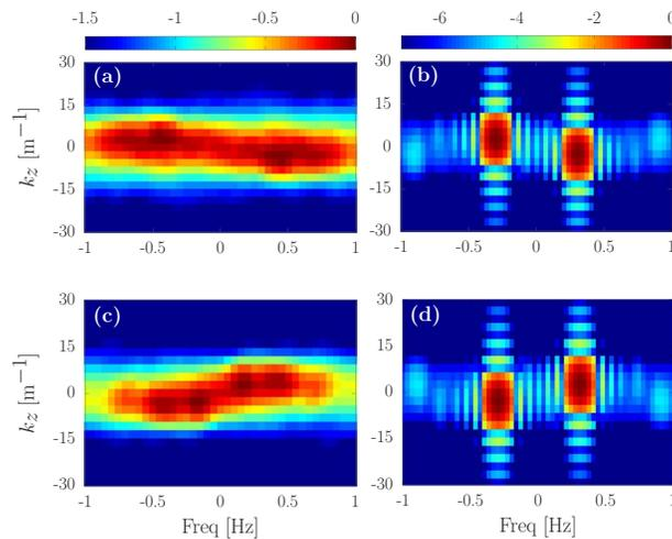
FIG. 6. Left, experimental spatio-temporal spectrum  $E_E(k_z, f)$  for (a)  $\theta = 0$ ,  $\text{Re} \approx 10^6$  and (c)  $\theta = -8 \times 10^{-3}$ ,  $\text{Re} \approx 8 \times 10^5$ . Right, synthetic spatio-temporal spectrum  $E_S(k_z, f)$  with  $n = k/k_0 = 1$ ,  $m = 3$  and using (b)  $f_v = 0.1$  Hz and (d)  $f_v = -0.1$  Hz. Colors are log scaled.
