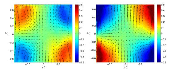
FIG. 2. Structure of the mean velocity field for  $\theta = 0$ . The arrows represents directions and intensities of the velocity components in the PIV plan averaged over time  $(\bar{u}, \bar{v})$ . The orthogonal component  $\bar{w}$  is represented by the color scale. Left: (+) sense of rotation. Right: (-) sense of rotation.
