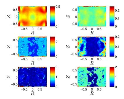
FIG. 4. ARMA analysis for the (+) sense of rotation. Top left:  $|\vec{V}|$ . Top right:  $|\vec{V}(t)|$  standard deviation. Center left: Total order  $\mathcal{O}$  found by fitting an ARMA(p,q) to the  $|\vec{V}(t)|$  data. Center right: Distance from the Kolmogorov model  $\Upsilon$  for the  $|\vec{V}(t)|$  data. Bottom left: Sum of the autoregressive coefficient  $\Phi$ . Bottom right: Sum of the moving average coefficients  $\Theta$ .
