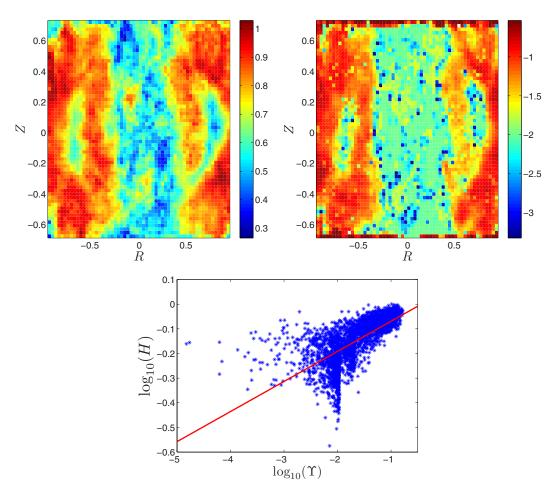
FIG. 8. Upper panels: Comparison between the Hurst exponents H (left) and the deviation from the Kolmogorov model in log-scale  $\log_{10}(\Upsilon)$  (right) found by fitting an ARMA(p,q) to the  $|\vec{V}(t)|$  data for the (+) sense of rotation. Lower panel: Scatter plot of the Hurst Exponent H and  $\log_{10}(\Upsilon)$ . The red solid line shows a linear fit to the data.
