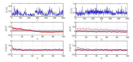
FIG. 3. Two time series of |V(t)| (upper panels) with their respective ACF functions (middle panels) and PACF (lower panels).  $Re \simeq 10^5$ , (+) sense of rotation. Blue lines in the ACFs and PACFs represent the confidence bands at the 95% confidence level. Sample frequency: 15 Hz. X-axis is in sample index.
