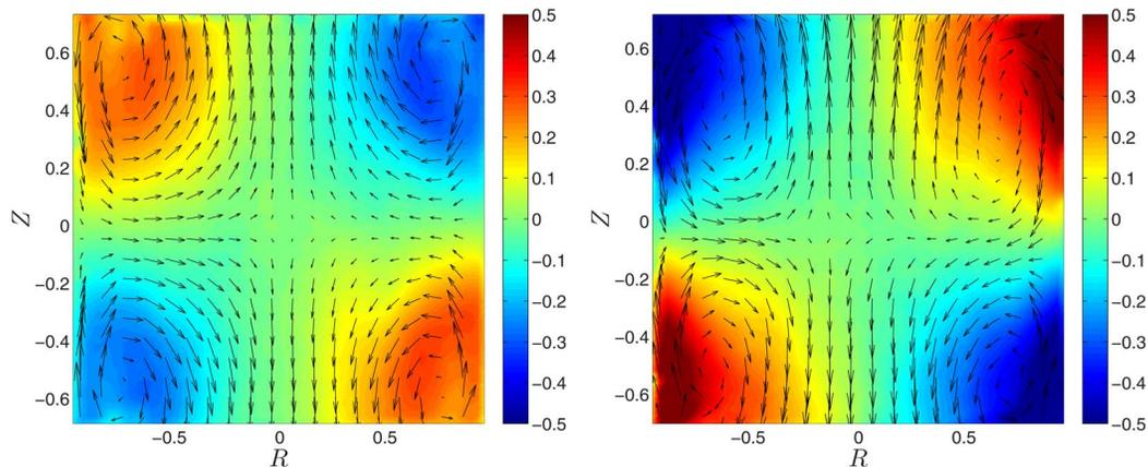
FIG. 2. Structure of the mean velocity field for  $\theta = 0$ . The arrows represent directions and intensities of the velocity components in the PIV plane averaged over time ( $\bar{u}$ ,  $\bar{v}$ ). The orthogonal component  $\bar{w}$  is represented by the color scale. Left: (+) sense of rotation. Right: (−) sense of rotation.
