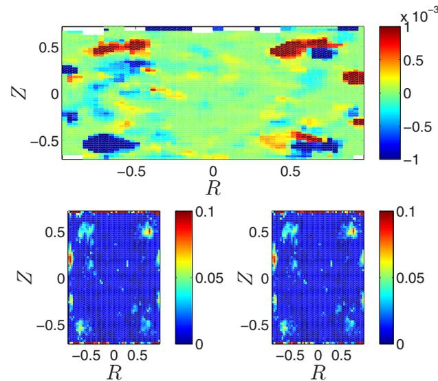
FIG. 7. Upper panel: Difference between  $\Upsilon$  computed for the  $|\vec{V}(t)|$  data for the (–) sense of rotation and  $\Upsilon$  on surrogate data of the same experiment obtained with a phase randomization procedure. Lower panel:  $\Upsilon$  for the original data (left) and for the surrogates (right).
