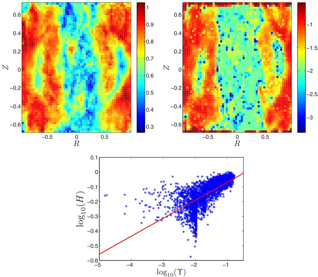
FIG. 8. Upper panels: Comparison between the Hurst exponents  $H$  (left) and the deviation from the Kolmogorov model in log-scale  $\log_{10}(\Upsilon)$  (right) found by fitting an  $\text{ARMA}(p,q)$  to the  $|\vec{V}(t)|$  data for the (+) sense of rotation. Lower panel: Scatter plot of the Hurst Exponent  $H$  and  $\log_{10}(\Upsilon)$ . The red solid line shows a linear fit to the data.
