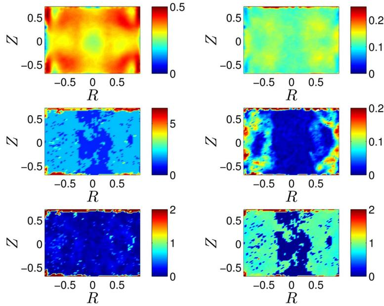
FIG. 4. ARMA analysis for the (+) sense of rotation. Top left:  $|\vec{V}|$ . Top right:  $|\vec{V}(t)|$  standard deviation. Center left: Total order  $\mathcal{O}$  found by fitting an ARMA( $p,q$ ) to the  $|\vec{V}(t)|$  data. Center right: Distance from the Kolmogorov model  $\Upsilon$  for the  $|\vec{V}(t)|$  data. Bottom left: Sum of the autoregressive coefficient  $\Phi$ . Bottom right: Sum of the moving average coefficients  $\Theta$ .
