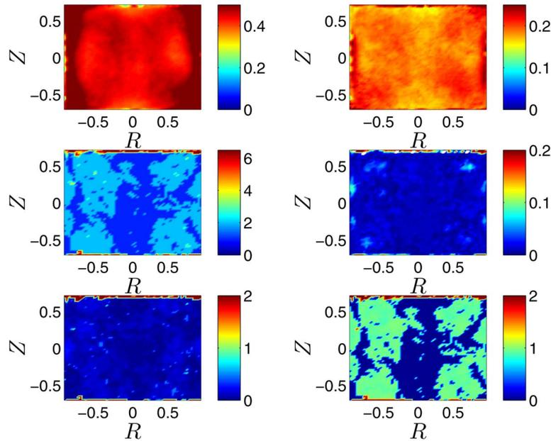
FIG. 5. ARMA analysis for the (-) sense of rotation. Top left:  $|\vec{V}|$ . Top right:  $|\vec{V}(t)|$  standard deviation. Center left: Total order  $\mathcal{O}$  found by fitting an ARMA( $p,q$ ) to the  $|\vec{V}(t)|$  data. Center right:  $\Upsilon$  for the  $|\vec{V}(t)|$  data. Bottom left: Sum of the autoregressive coefficient  $\Phi$ . Bottom right: Sum of the moving average coefficients  $\Theta$ .
