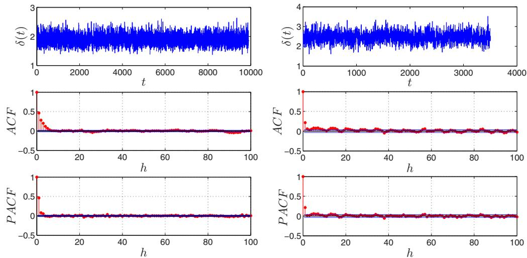
FIG. 9. Time series of  $\delta(t)$  (upper panels) with their respective ACF functions (middle panels) and PACF (lower panels). Left: (+) sense of rotation. Right: (-) sense of rotation.  $Re \simeq 10^5$ . Blue lines in the ACFs and PACFs represent the confidence bands at the 95% confidence level. Sample frequency: 15 Hz. X-axis is in sample index.
