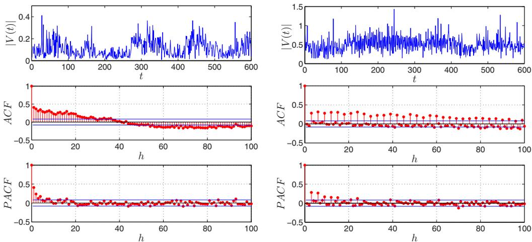
FIG. 3. Two time series of  $|V(t)|$  (upper panels) with their respective ACF functions (middle panels) and PACF (lower panels).  $Re \simeq 10^5$ , (+) sense of rotation. Blue lines in the ACFs and PACFs represent the confidence bands at the 95% confidence level. Sample frequency: 15 Hz. X-axis is in sample index.
