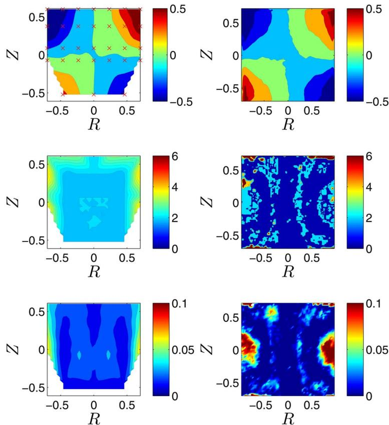
FIG. 6. Comparison between the ARMA analysis for LDV data (left) and PIV data (right) for the azimuthal component of the velocity  $w$ .  $\bar{w}$  (upper panels), total order  $\mathcal{O}$  (central panels) and distance from Kolmogorov model  $\Upsilon$  (lower panels); (–) sense of rotation;  $Re \simeq 10^5$ . The red crosses in the top-left panel show the locations of the measurement points for the LDV experiment.
