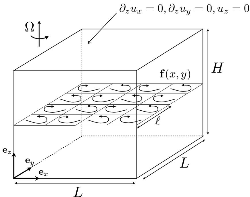
FIGURE 1. Flow of a Newtonian fluid in a frame rotating at angular velocity  $\Omega$  around the vertical  $z$  axis. It is driven by a horizontal body-force  $\mathbf{f}$  that is independent of the vertical. We assume periodic boundary-conditions in the horizontal, and stress-free boundaries at  $z = 0$  and  $z = H$ .
