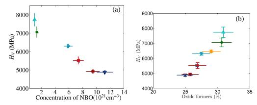
**Fig. 13.** (a) Evolution of hardness,  $H_V$  (at 50 g in ambient conditions), versus the concentration of non-bridging oxygen (NBO) deduced from NMR measurements. (b) Evolution of hardness,  $H_V$  (at 50 g in ambient conditions), versus percentage of oxide formers determined from ICP measurements.
