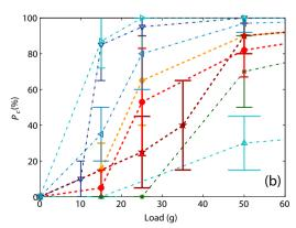
**Fig. 8.** (a) Crack appearance probability for all the SBN glasses  $K_{SBN} = 2.1$  series (blue) and  $K_{SBN} = 3.7$  series (red) at different loads. (b) A zoom of the crack appearance probability for all the SBN glasses  $K_{SBN} = 2.1$  series (blue) and  $K_{SBN} = 3.7$  series (red) for loads between 0 g and 50 g.
