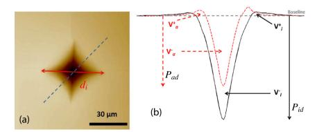
**Fig. 1.** (a) A typical indentation imprint used to determine the indentation diagonal length, ( $d_i$  and marked by a continuous line) and to estimate the pile-up profile (dotted line). (b) Sketch showing the evolution of indentation prints before (black solid line) and after annealing (red dotted line).  $V^+$  and  $V^-$  represent the volume above and below the baseline (gray dotted line), respectively.
