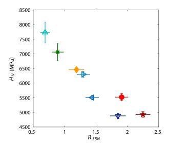
**Fig. 6.** Hardness values,  $H_V$ , versus  $R_{\rm SBN}$  for SBN glasses (at 50 g during 15 s in ambient conditions).
