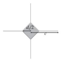
**Fig. 2.** Sketch of a Vickers's indent and notations used to define  $K_C^{VIF}$ :  $d_i$  is the indentation diagonal length from one indent and  $c_i$  is the crack length measured from the indentation center.
