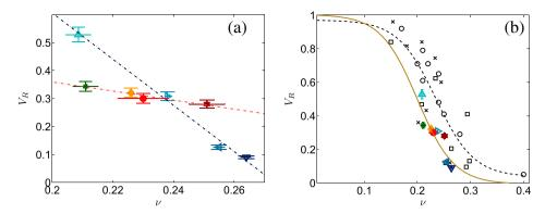
Fig. 18. (a) The figure depicts the evolution the volume recovery ratio  $(V_R)$  versus the Poisson's ratio  $(\nu)$  for SBN data. The blue color line depicts a linear fit to the data for  $K_{\rm SBN} \sim 2.5$   $(V_R = m_{K_{\rm SBN} \sim 2.5} \nu + b_{K_{\rm SBN} \sim 4.5} \nu + b_{K_{\rm SB$
