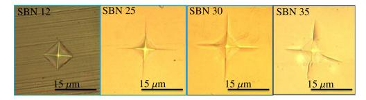
**Fig. 4.** Evolution of indentation prints for the  $K_{SBN} \sim 2.5$  series (from left to right: SBN 12, SBN 25, SBN 30, and SBN 35) at 50 g in ambient conditions. An optical camera coupled with the Vickers's indenter captures the imprints within 5 min after indentation.
