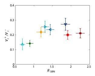
**Fig. 11.** The normalized ratio  $(V_i^+/V_i^-)$  of the glasses pile-up with  $R_{\rm SBN}$  displays two trends depending on  $K_{\rm SBN}$ . For  $K_{\rm SBN} \sim 2.5$ , the ratio increases initially then appears to stabilize. For  $K_{\rm SBN} \sim 4.5$ , the ratio decreases slightly.
