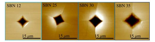
Fig. 5. Evolution of indentation prints for the  $K_{SBN} \sim 2.5$  series (from left to right: SBN 12, SBN 25, SBN 30, and SBN 35) at 50 g in ambient conditions. An AFM scans the indents after indentation.
