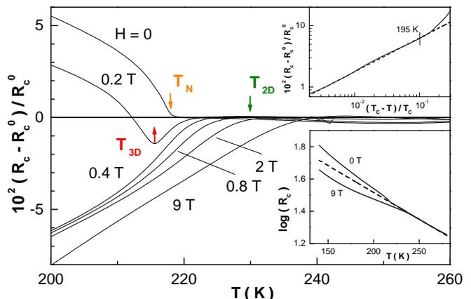
FIG. 1:  $c$ -axis resistance anomaly, as obtained subtracting a high temperature linear logarithmic resistance (dashed line in lower inset). Upper inset: scaling of the resistive anomaly. The magnetic field is applied along the  $c$ -axis.
