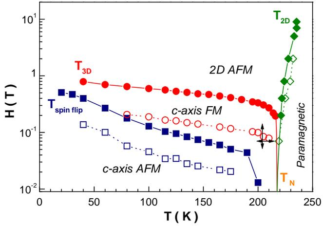
FIG. 2: Phase diagram for the transverse resistivity, as obtained from the data in Fig. 3 (squares and circles) and the onset in Fig. 1 (diamonds). Filled symbols are for field applied along the  $c$ -axis; open ones, in the  $a$ - $b$  plane.  $T_N$  is the zero field transition temperature, as given by the data in Fig. 1.
