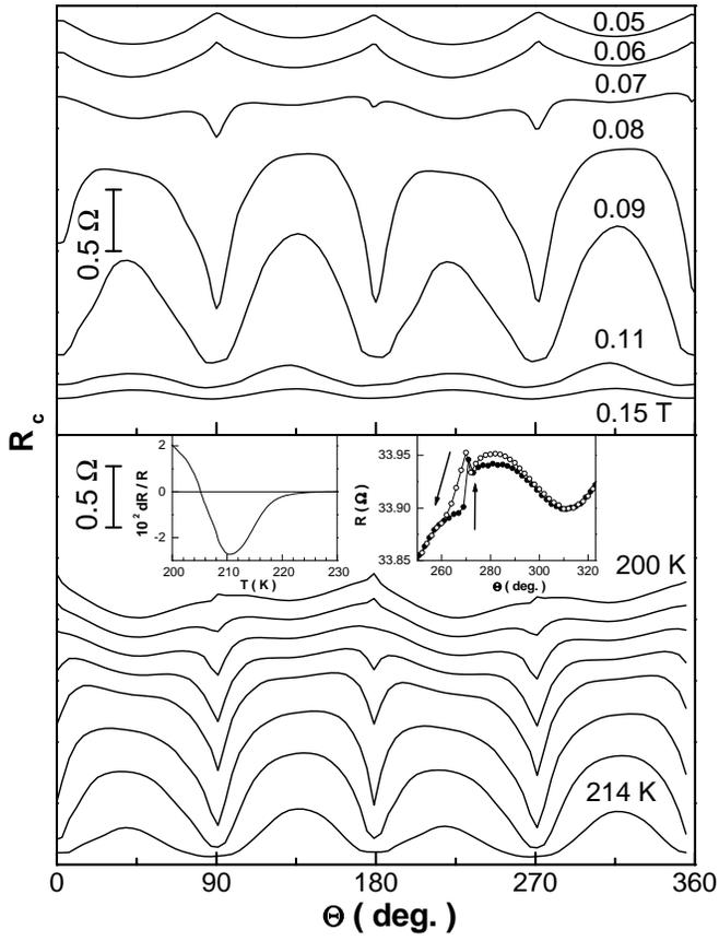
FIG. 7: Angular dependence of the magnetoresistance along the two segments in Fig. 2 (field in the  $a$ - $b$  plane). Upper panel:  $T = 204$  K. Lower panel:  $H = 0.07$  T ( $T$  varies in steps of 2 K); left inset: resistance anomaly in zero field, obtained as in Fig. 1; right inset: occurrence of a uniaxial hysteretic feature ( $T = 200$  K).
