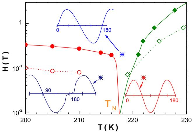
FIG. 4: Torque ( $\Gamma$ ) angular dependence at typical locations in the  $H$ - $T$  plane. Magnetic field is rotated in the  $a(b)$ - $c$  plane. The angle is the one from the  $c$ -axis. Symbols are from Fig. 2.
