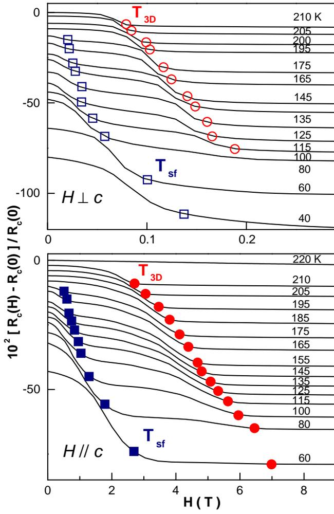
FIG. 3:  $c$ -axis magnetoresistance, for field along (lower panel) and perpendicular to  $c$ -axis (upper). Symbols mark the characteristic fields in Fig. 2. (curves have been shifted from their  $H = 0$  zero value, for clarity)
