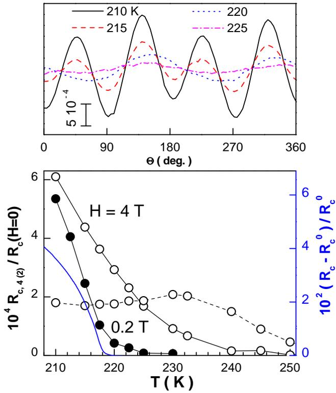
FIG. 5: Upper panel: angular dependence of the magnetoresistance (in-plane field  $H = 0.2$  T);  $\theta$  is the angle between  $a(b)$  and the magnetic field. Lower panel: Symbols: four-fold and two-fold (dotted line) components of the angular  $c$ -axis magnetoresistance (left scale). Full line: zero field  $c$ -axis resistance anomaly, as in Fig. 1
