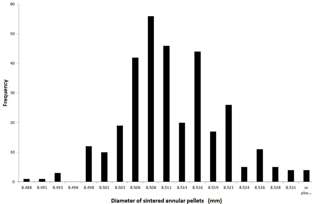
**Fig. 4.** Histogram of the sintered pellet diameter.
