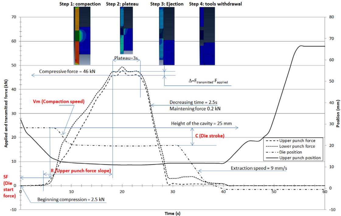
**Fig. 1.** Upper, applied and lower transmitted punch forces, die and upper punch displacements depending on time, Von Mises stresses during step calculations (1 to 4), corresponding to the compaction cycle.
