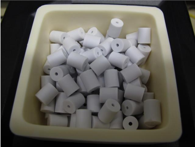
**Fig. 3.** Sintered pellets in the alumina container (100 pellets).
