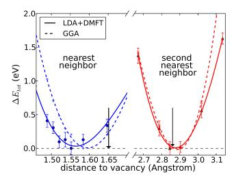
FIG. 5: Total energy vs distance to the vacancy for the first nearest neighbor (blue) and the second nearest neighbor (red), in DFT+DMFT (full line) and GGA (dashed line). The black arrows show the position of the atoms in the unrelaxed bcc supercell. (Colors online)
