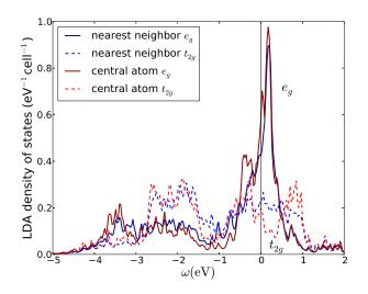
FIG. 6: Density of states on the  $e_g$  (full line) and  $t_{2g}$  (dashed line) on the first nearest neighbor to the vacancy (blue) and on the central atom (red). (Color online)
