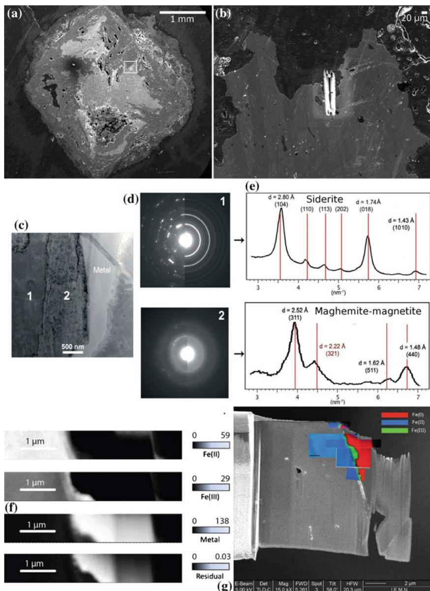
**Fig. 3** a SEM image of the cross section of an archaeological iron nail corroded since the 15th c. in an anoxic carbonated environment. b Location of the thin film sample at the metal/corrosion product interface, c TEM image and associated (d, e) electron diffraction patterns. (f, g) STXM maps obtained at the Fe L edge. Repartition of Fe(0), Fe(II) and Fe(III) valences (Michelin et al. 2013; Leon et al. 2014)
