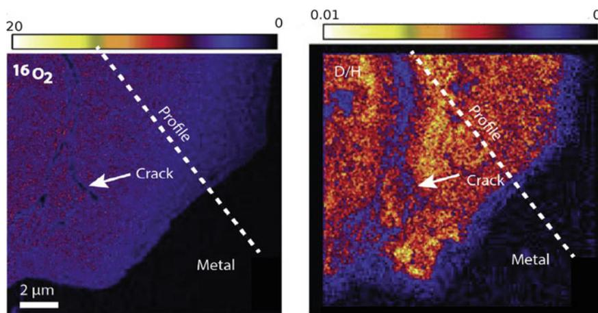
**Fig. 4** Nano-SIMS maps of  $^{16}O_2$  and D/H ratio obtained at the Metal/Corrosion products interface of an archaeological nail from the 15th c. put 3 month in a  $D_2O$  solution (Leon et al. 2014)
