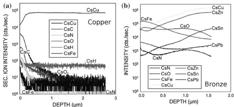
**Fig. 9** **a** Normalised D-SIMS depth profile on a copper sample after presenting a 200 nm reddish brown nitrate solution patina, **b** Normalised D-SIMS depth profile on a bronze sample after presenting a 1600 nm reddish brown nitrate solution patina (Balta et al. 2009)
