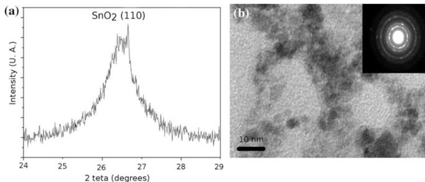
**Fig. 7** **a** XRD at incidence angle  $\gamma = 5^\circ$  of  $\text{SnO}_2$  powder separated from the surface of a corroded Andalusian baroque mirror by the sonication method **b** TEM image and electron diffraction patterns from  $\text{SnO}_2$  particles from the surface of a corroded mirror (Herrera et al. 2009)
