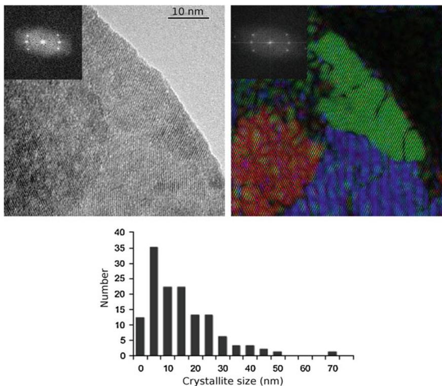
**Fig. 2** HR-TEM images of goethite from the corrosion products taken on the reinforcing chain of the triforium of the Amiens cathedral (15th c.), corresponding Fourier transformed image and crystallite sizes (Monnier et al. 2010b)
