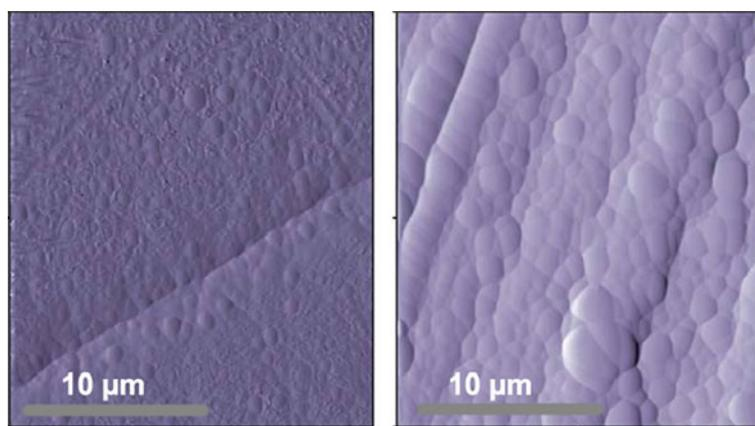
**Fig. 11** AFM images of SiO<sub>2</sub>-like films deposited by PECVD on copper based reference alloys of different roughness, representative of metals of cultural heritage (Angelini et al. 2006)
