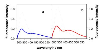
**Figure 4.** Comparison of the fluorescence spectra of the duplexes (solid lines) n-ds and m-ds with those of the corresponding stoichiometric mixture of nucleosides (dots); (a, blue) non-methylated systems; (b, red) methylated systems. The spectral intensities are representative of the fluorescence quantum yields. Excitation wavelength: 255 nm.
