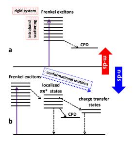
**Figure 9.** Effect of the duplex rigidity on the intraband scattering and its consequence to CPD formation. In rigid systems (a), intraband scattering leads to the bottom of the exciton band, transferring the excitation energy to reactive bases. In the presence of conformational motions (b), intraband scattering is in competition with localization
