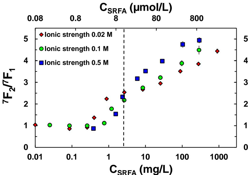
Figure 2. Evolution of  ${}^5\text{D}_0 \rightarrow {}^7\text{F}_2 / {}^5\text{D}_0 \rightarrow {}^7\text{F}_1$  area ratios vs.  $C_{\text{SRFA}}$  the ionic strength ( $I = 0.02$  M, red diamonds;  $I = 0.1$  M, green circles;  $I = 0.5$  M, blue squares) at  $C_{\text{Eu(III)}}$  of  $1 \mu\text{M}$  and pH 7. Dashed line corresponds to the inversion of the ionic strength trend.
