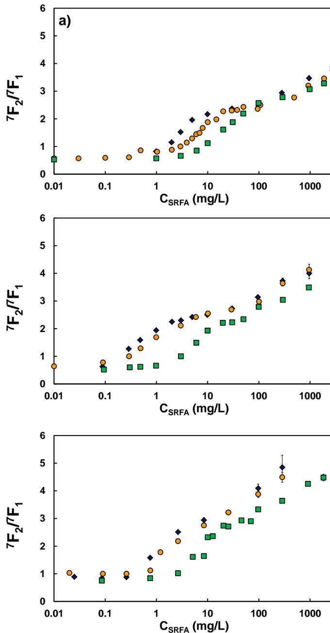
Figure 1. Evolution of  ${}^5D_0 \rightarrow {}^7F_2 / {}^5D_0 \rightarrow {}^7F_1$  area ratios  $w$ .  $C_{\text{SRFA}}$  at  $I = 0.1$  M, pH 4 (a); pH 6 (b), and pH 7 (c) for  $C_{\text{Eu(III)}}$  of 0.5 (blue diamonds), 1 (orange circles), and 10  $\mu\text{M}$  (green squares):  $\lambda_{\text{exc}} = 393.7$  nm,  $D = 10$   $\mu\text{s}$ ,  $W = 300$   $\mu\text{s}$ , 600 lines. $\text{mm}^{-1}$  grating. Error bars represent  $2\sigma$  of the area ratio using the trapezoid method.
