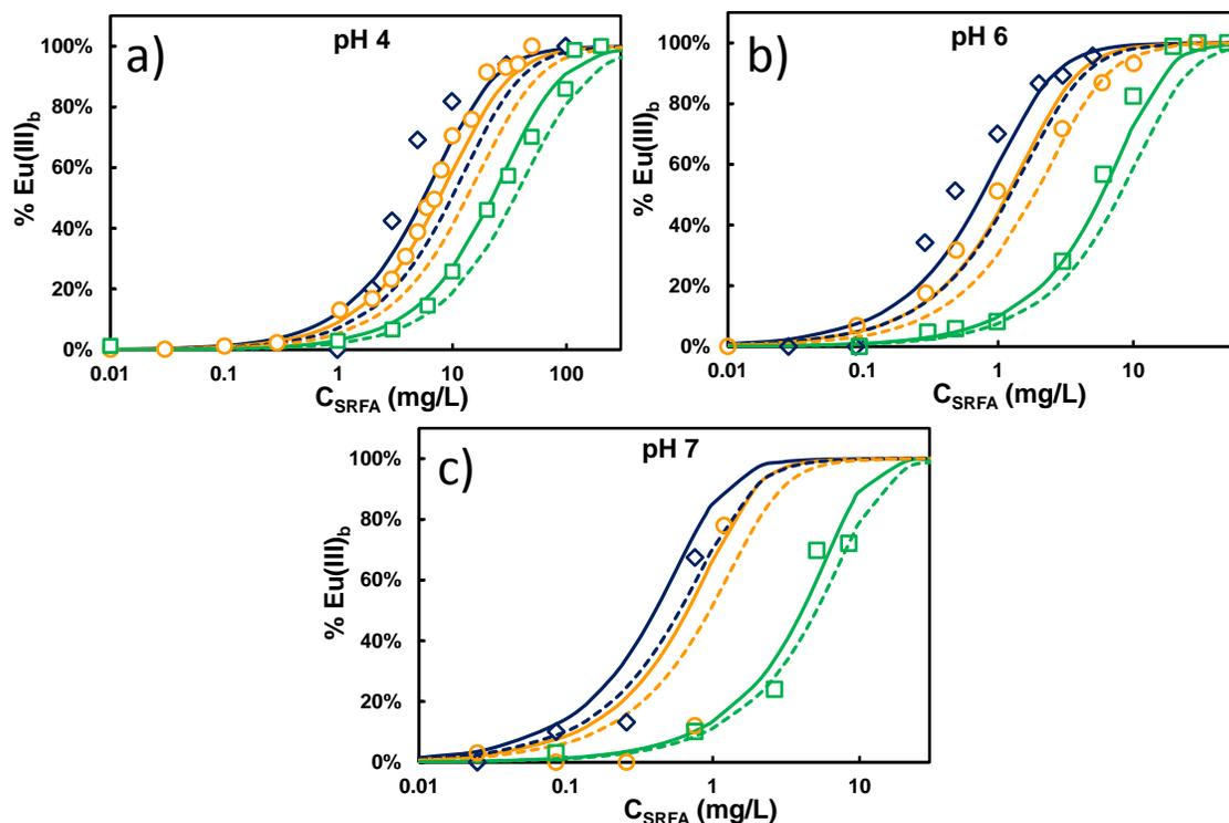
Figure 3. Proportion of Eu(III) bound to SRFA for Eu(III) concentrations of 0.5  $\mu\text{M}$  (blue diamonds), 1  $\mu\text{M}$  (orange circles) and 10  $\mu\text{M}$  (green squares) at pH 4 (a), 6 (b), and 7 (c). The dashed lines are the simulations and the solid lines are the results of our modeling of Eu(III) bound to SRFA. Adjusted and generic NICA Donnan parameters are given in Table S1 of the SI.
