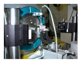
**Figure 1.** Setup for pulse radiolysis at GANIL (Experiment n°P492 on 19<sup>th</sup> of June 1999). Center of the picture: a vertical optical cell made of fused silica is irradiated with horizontal beam downstream the output "nose" of the machine made of a thin titanium foil.
