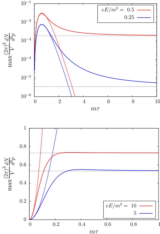
Figure 18: Plots of the maximum value of the momentum spectrum as a function of  $m\tau$  for several values of  $eE/m^2$ . Top: subcritical field strength  $eE/m^2 < 1$ . Bottom: supercritical field strength  $eE/m^2 > 1$ . The all-order exact result (124) (solid lines) and the lowest-order perturbative result (239) (dashed lines) are compared. The constant field Schwinger result  $\exp(-\pi m^2/(eE))$  is plotted as thin black lines.
