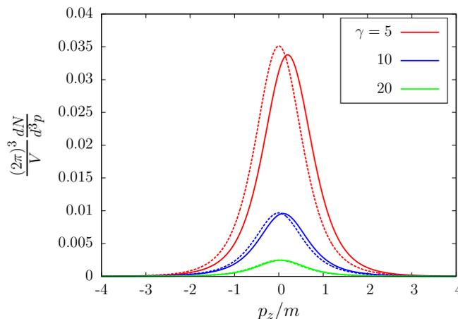
Figure 17:  $p_z$ -dependence of the spectrum at  $p_{\perp} = 0$ . The all-order exact result (124) (solid lines) and the lowest-order perturbative result (239) (dashed lines) are compared for several values of the Keldysh parameter  $\gamma$ . The ratio  $eE/m^2 = 1$  is fixed. For  $\gamma = 20$ , the two lines are almost undistinguishable.
