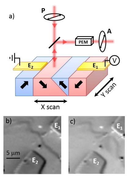
**Figure 2**:a) Schematics of the optical measurement where a focused laser spot is scanned on the sample and two quantities are recorded including the change of light polarization and the current extracted through the electrodes. The latter allows to map the photocurrent generation while the former gives the ferroelectric domain configuration as shown on the two images (b and c) where the dark line corresponds to the domain wall.
