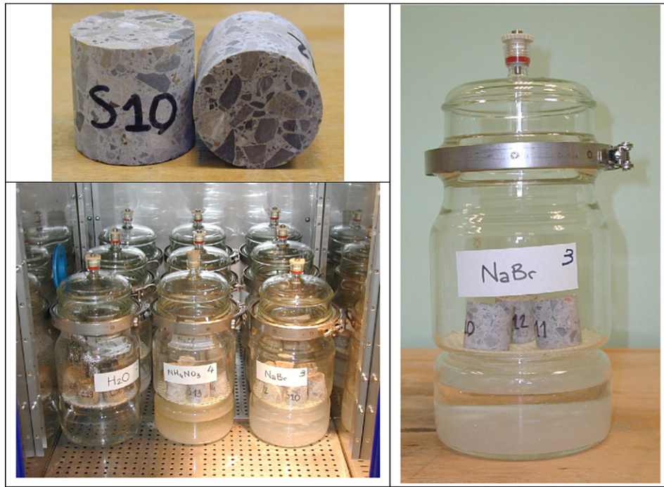
Fig. 3. View of the 40 mm × 40 mm samples and the climatic boxes containing the saturated salt solutions. Note the opening at the top of the containers which allows inserting a probe for verification of both temperature and RH.
