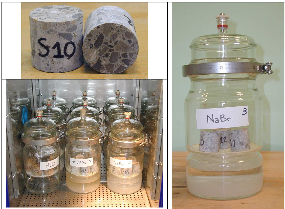
155 Fig. 3. View of the 40 mm x 40 mm samples and the climatic boxes containing the saturated 156 salt solutions. Note the opening at the top of the containers which allows inserting a probe for 157 verification of both temperature and RH.
