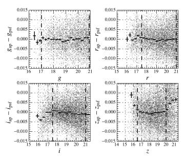
**Fig. 1.** Difference between aperture and PSF photometry as a function of the SNLS tertiary standard star magnitude. The aperture photometry from B13 has been corrected for residual contamination using an estimate of the local background level obtained with PSF photometry. The magnitude range used in the zero-point fit (vertical dashed lines) is chosen so that the aperture catalog is expected to be free from selection bias (B13, Fig. 12).
