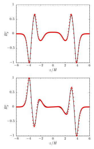
**Fig. 4.** Comparison of  $B_y(z)$  from the simulation (red circles) and from the linear calculation (black line), which include Ohmic and Hall diffusion computed at 1 au with  $\beta_0 = 10^5$ . *Top:* n = 1 eigenmode and symmetric component of  $B_y(z)$ . *Bottom:* n = 2 eigenmode and antisymmetric component of  $B_y(z)$ .
