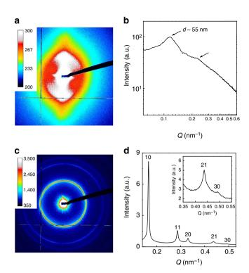
**Figure 5 | SAXS measurements of SW Si-INT suspensions.** SAXS patterns of **(a)** nematic ( $\phi = 0.14\%$ ) and **(c)** columnar ( $\phi = 0.31\%$ ) SW Si-INT suspensions and **(b,d)** their corresponding *I*(*Q*) curves. (The hk indices in **d** refer to the 2D hexagonal reciprocal lattice peaks.)
