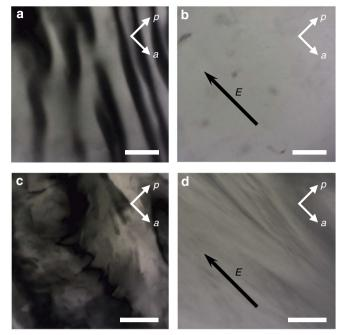
Figure 6 | Texture photographs of aligned imogolite suspensions. (a,b) nematic ( $\phi = 0.12\%$ ) and (c,d) columnar ( $\phi = 0.22\%$ ) DW Ge-INT suspensions before (a,c) and after (b,d) application of an electric field  $E = (100 \text{ V mm}^{-1}, 500 \text{ kHz})$ . Scale bar, 100 µm.
