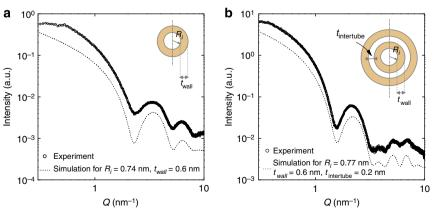
Figure 1 | WAXS measurements of imogolite nanotubes. Experimental (open circles) and calculated (dotted line) WAXS curves of (a) SW Si-INT and (b) DW Ge-INT in suspension. The insets represent sketches of a single-walled and a double-walled nanotube. For the sake of clarity, calculated curves (using equations (1) and (3)) have been translated vertically.
