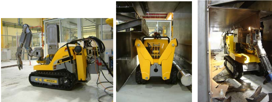
Figure 7: a) Brokk 90 equipped with an on-board controller and the Cybernétix Maestro arm; b) the machine in the technical gallery mock-up; c) in action with a nibbler.
