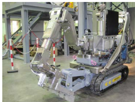
Figure 8: Cybernétix industrial version of a Brokk 90 equipped with an on-board controller and the Maestro arm. Tool rack on the front of the machine.
