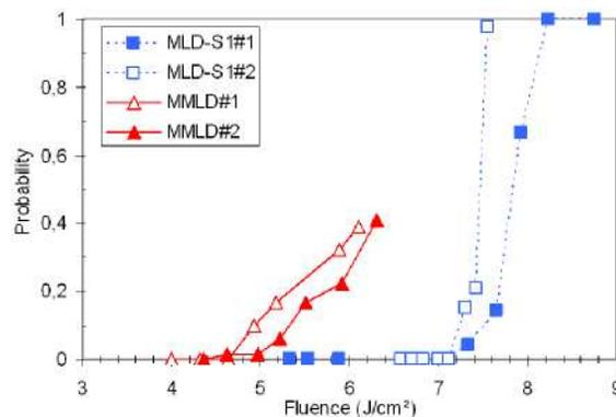
Fig. 4. Damage probability curves obtained after laser irradiation of different samples at  $1057\text{nm}$ ,  $500\text{fs}$ , TE polarization. MLD are tested at an incidence of  $77.2^\circ$ , MMLD are tested at  $72^\circ$ . No angular correction is made.
