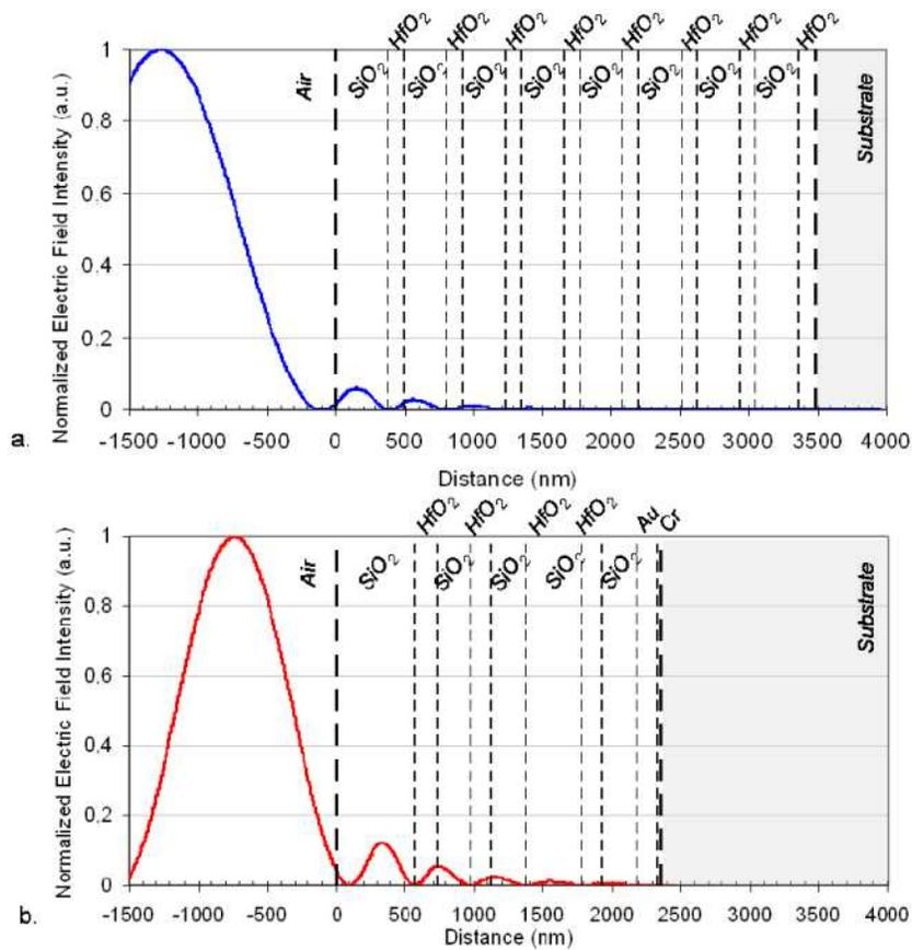
Fig. 5. Electric field distribution of the MLD (a) and the MMLD (b) samples. EFI is calculated and plotted in the damage testing conditions i.e.  $72^\circ$  for the MMLD and  $77.2^\circ$  for the MLD.
