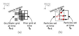
Figure 3: (a) Prior grids propagation. (b) Particles propagation.
