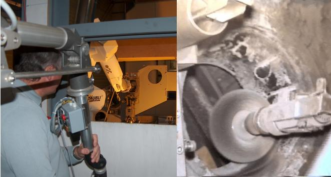
Fig. 8. Brushing task on the mock up (left) and in the hot cell (right).
