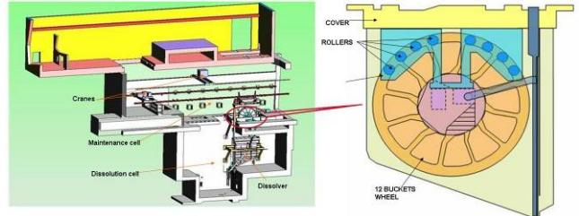
Fig. 6. CAD model of the dissolution cell and wheel.
