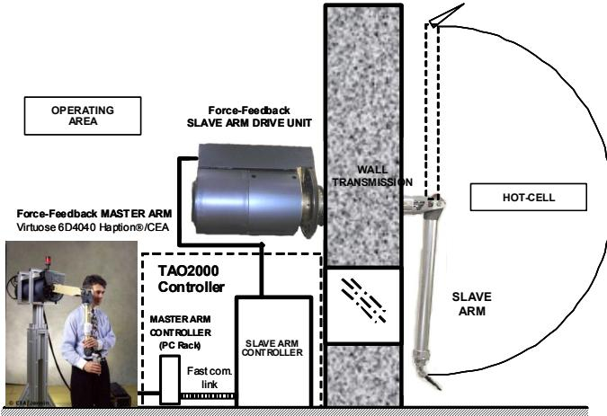
Fig. 4. Hardware architecture of a MT200 TAO based AREVA CAT system
