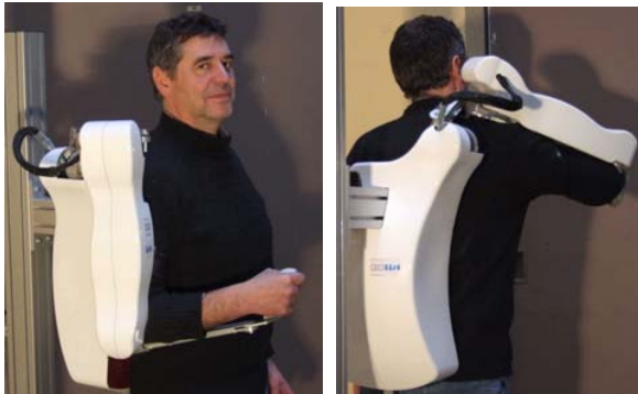
Fig 1. ABLE 4 axis exoskeleton actuated by screw-and-cable actuators
