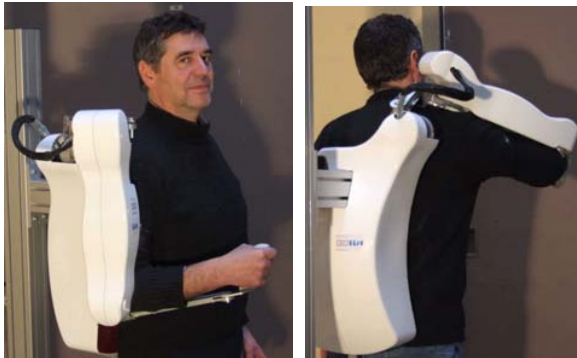
Fig 1. ABLE 4 axis exoskeleton actuated by screw-and-cable actuators
