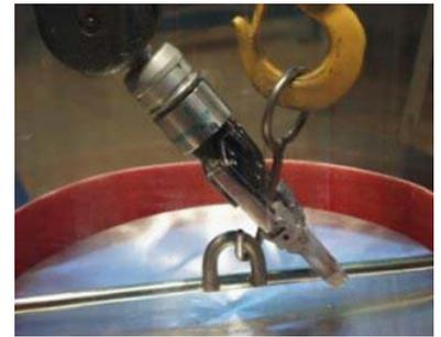
Figure 11 : Securing a hook on the handling bar
