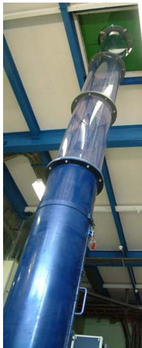
Figure 26 : Mockup of an interim storage shaft
