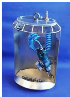
**Figure 21 : Pod for installing a lifting bar using threaded anchoring points**
