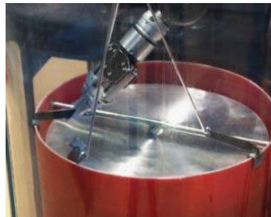
Figure 10 : Installing a lifting bar
