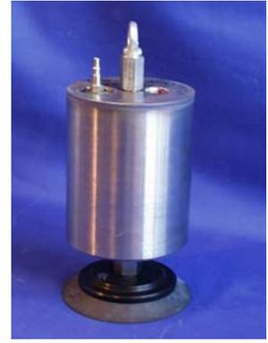
Figure 25 : Tool for recovery of small flat objects
