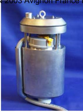
Figure 23 : Powder vacuuming pod
