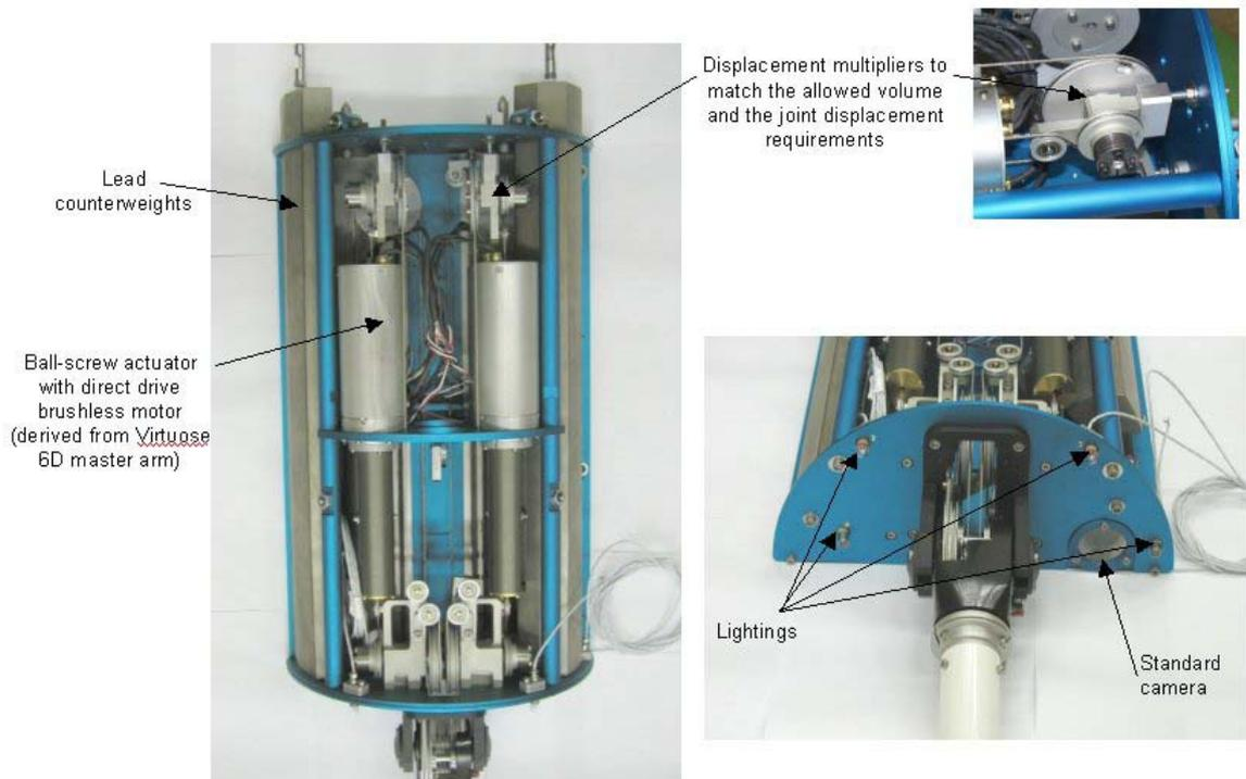
Figure 18 – Slave actuator unit of the prototype
