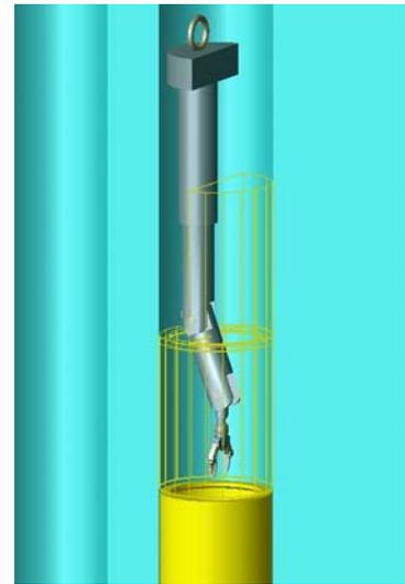
**Figure 4 : Arm with 5 DoF (Translation-Roll-Pitch-Pitch-Roll)**
