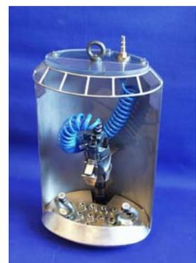
**Figure 22 : Pod for installing and removing the screw-on cover of a waste container**
