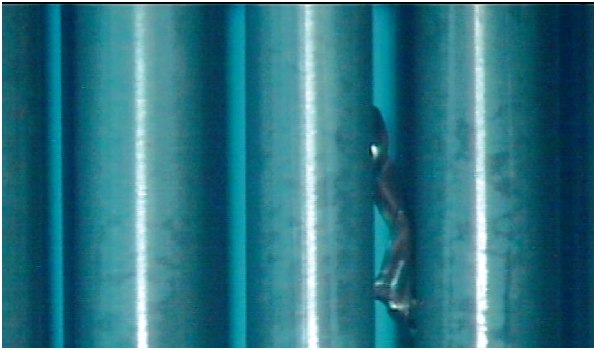
Fig. 20. Debris trapped between two rows of fuel rods in a PWR assembly.
