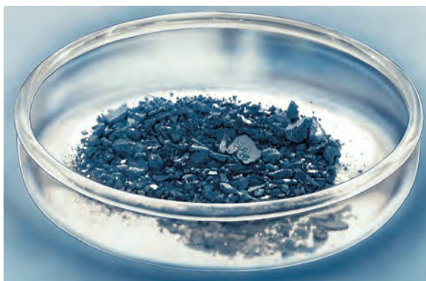
Fig. 37. Mo-Zr deposits, sampled from a dissolver in the UP3 plant, La Hague.
