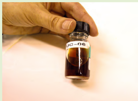
Fig. 97. Dissolution solution yielded by dissolution of uranium carbide by concentrated nitric acid at boiling point, with final composition: [U] = 50 \text{ g/l} , [HNO_3] = 5 \text{ M} .
