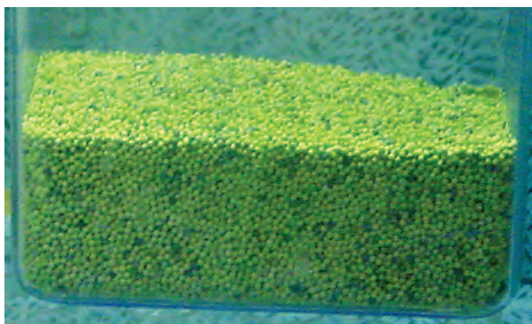
Fig. 40. Iodine-charged (yellow) solid sorbant, sampled from an industrial filter in the UP3 plant, at La Hague, after six years' operation.
