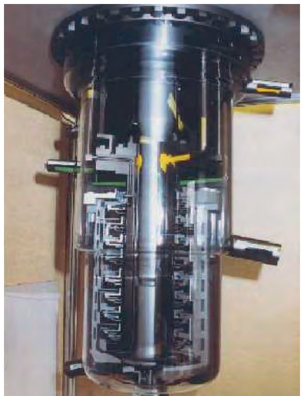
Fig. 58. Cutaway view of a Robatel centrifugal extractor, as used at the La Hague plant.
