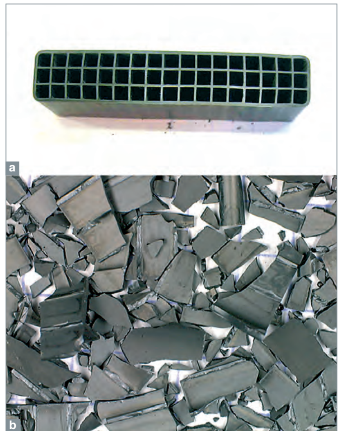
Fig. 95. View of a SiC honeycomb-cell macrostructured plate, prior to pulsed-current treatment (a), and after 1 pulse (b).
