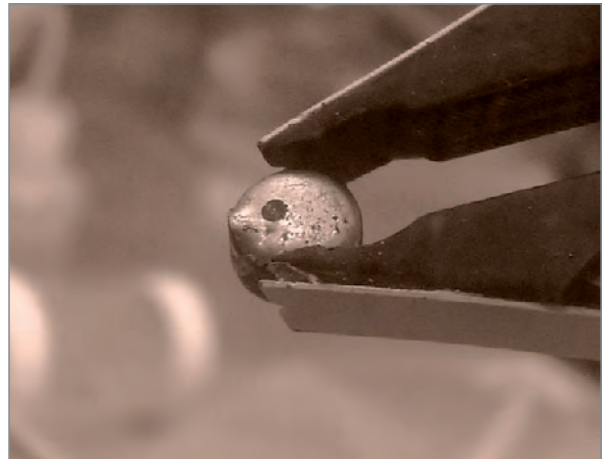
Fig. 170. Americium-loaded cadmium cathode (test carried out in the C10 line, in the ATALANTE facility).
