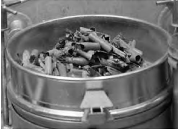
Fig. 30. Photograph of metallic components recovered at the UP3 plant, at La Hague (France), subsequent to shearing, and dissolution of PWR UOX fuel.
