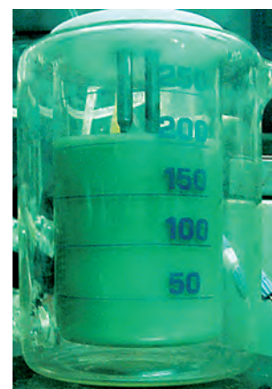
Fig. 150. Synthesis, at the scale of 1 gram or so, of a mixed U–Pu–Np–Am (78/20/1/1) oxalate in ATALANTE.
