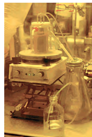
Fig. 149. Coconversion of Pu(IV)–Am(III) into oxide form in the ATALANTE facility.
