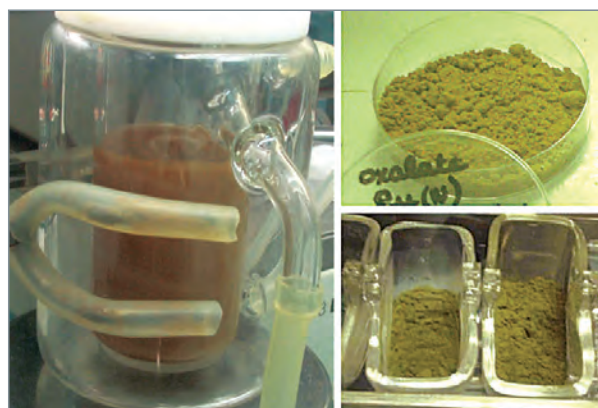
Fig. 65. Oxalic conversion of Pu(IV) into oxide: laboratory-scale tests; left: the vortex precipitation reactor; right (top): washed oxalate precipitate; right (bottom): the PuO 2 conversion product, subsequent to calcination.
