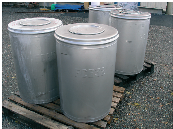
Fig. 74. Bituminized packages removed from the concrete container after corner drop test.
