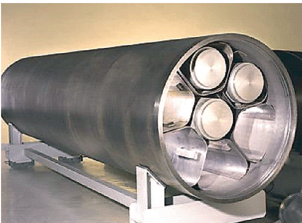
Fig. 145. Scale-1 demonstrator of the storage container for 7 spent fuel assemblies.
