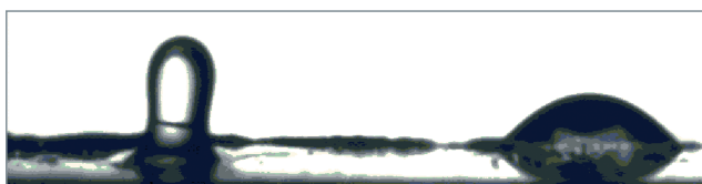
Fig. 8. A TBP drop as it is being detached from the film: by emulsification (left), and by roll-up (right).
