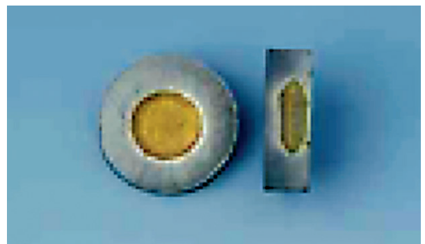
Fig. 109. Photograph of chopped pellets ( \text{Pb}_{10}(\text{VO}_4)_{4.8}(\text{PO}_4)_{1.2}\text{I}_2 ), in yellow, and ( \text{Pb}_3(\text{VO}_4)_{1.6}(\text{PO}_4)_{0.4} in grey), for iodine confinement.
