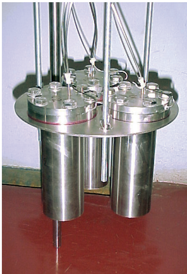
Fig. 79. "ERMITE" experiment: assembly of three 500-cm 3 mini-containers filled of cementitious material prior to being introduced into the irradiation device.
