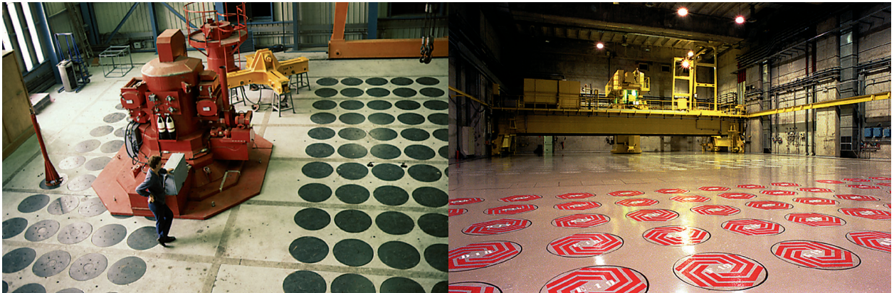
Fig. 24. Storage facilities at the CEA Marcoule Center (for claddings) and La Hague plant (for vitrified waste).
