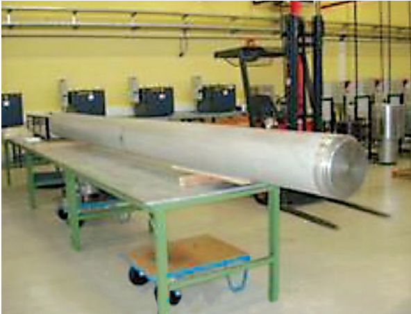
Fig. 144. Scale-1 demonstrator of the individual case for a spent fuel assembly.
