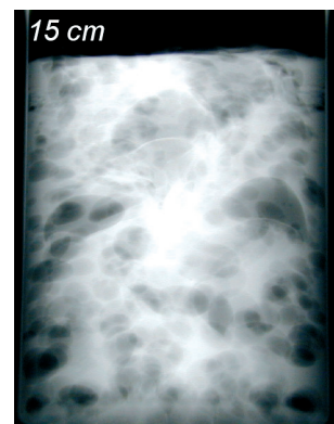
Fig. 88. X-radiographic cut of a synthetic bituminized waste which is subjected to an external gamma irradiation of about 1 MGy at 25 °C. Initially, the waste occupied half the experimental specimen.
