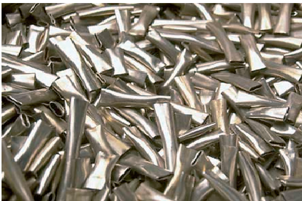
Fig. 95. Zircaloy-made cladding hulls.
