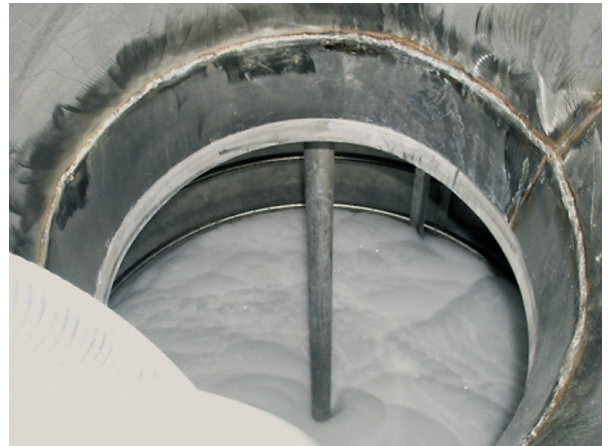
Fig. 7. Decontaminating foam in a tank contaminated by adhering deposits.
