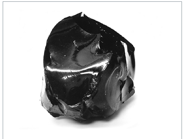
Fig. 19 a. Confinement glass block.
