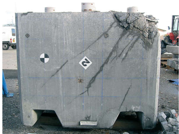
Fig. 73. Container B2.1 as resulting from a drop test, after lid removal.
