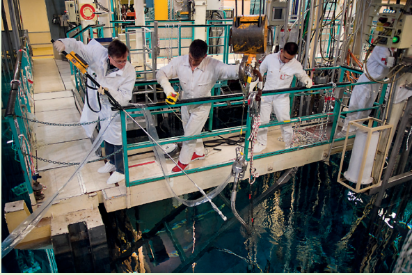
Fig. 75. The MERCI experiment: step of fuel transfer into the channel between the reactor and the hot cell.
