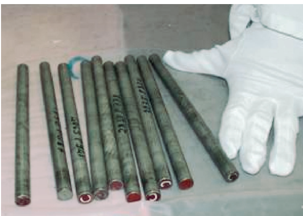
Fig. 52. Simulation element rodlets for the MASURCA core.
