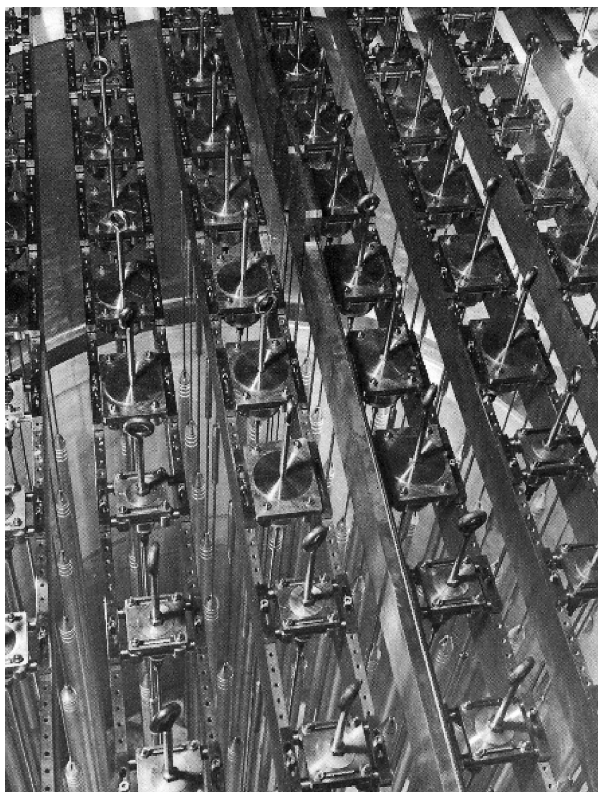
Fig. 24: AQUILON, a critical mockup used to qualify nuclear propulsion reactors.
