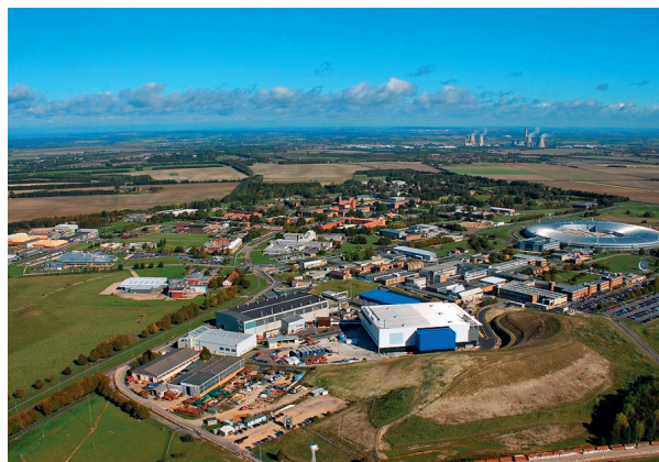
Fig. 15: Top view of ISIS, the English pulsed source located at the "Rutherford Appleton Laboratories" at Didcot, near Oxford. The two experimental halls can be seen in the foreground, each of them containing a different target.
