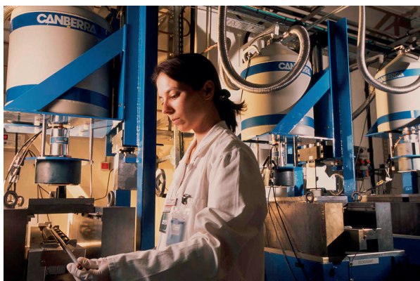
Fig. 41. Post-irradiation measurement on a fuel rod issued from the ÉOLE critical mockup.
