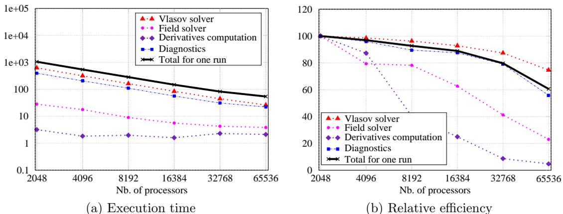
Figure 4: Strong scaling performed on the Curie machine from 2048 to 65536 cores: Execution time (a) and relative efficiency (b) for one GYSELA run of 4 iterations for a mesh  $(N_r \times N_\theta \times N_\varphi \times N_{v_{\sigma||}} \times N_\mu) = (512 \times 512 \times 128 \times 128 \times 32)$  with 8 threads and 32 values in  $\mu$  direction.
