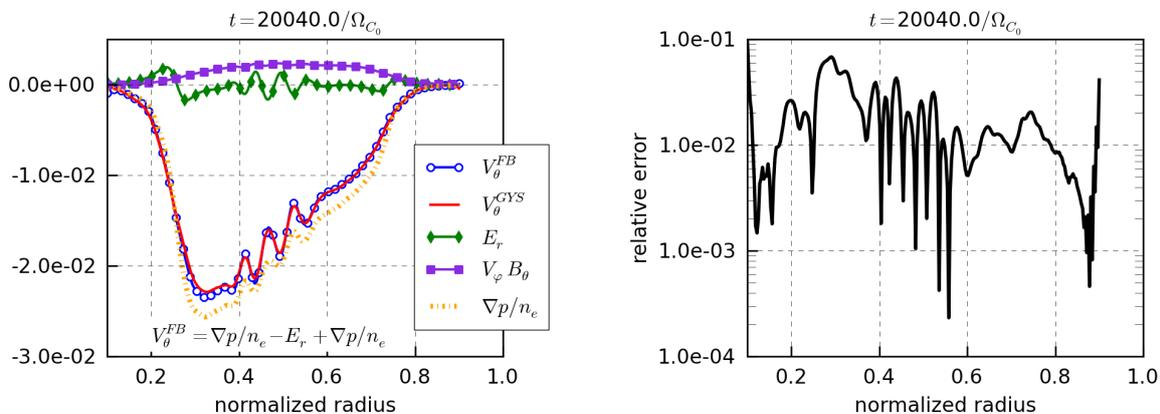
Figure 10: Left: Numerical test of the radial force balance equation (58) at time  $t = 20040\Omega_{C_0}^{-1}$ , comparing the poloidal velocity  $v_\theta^{\text{GYS}}$  directly computed in the code and  $v_\theta^{\text{FB}}$  the sum of the three contributions  $-E_r$ ,  $\nabla p / n_e$  and  $v_\varphi B_\theta$ . Right: Relative error between both. The parameters used for this simulation are summarized in Table 11.
