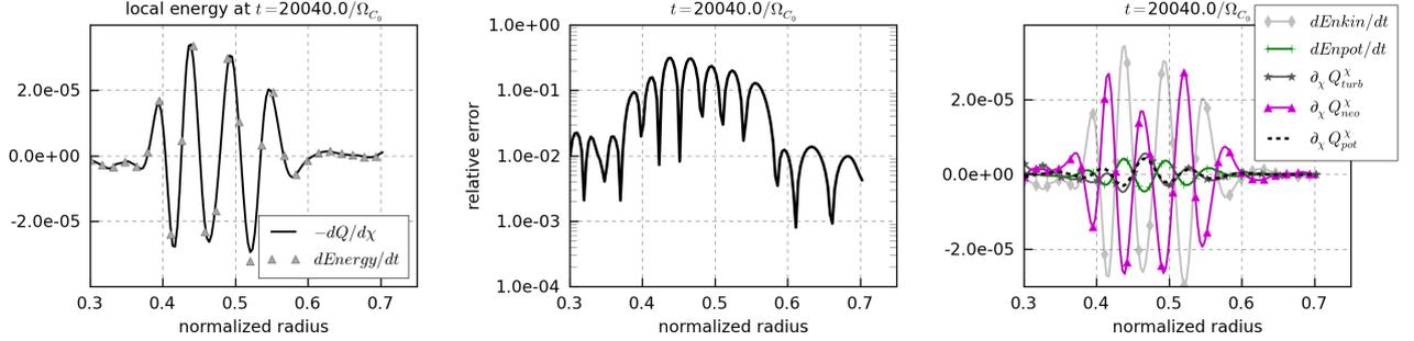
Figure 12: Numerical test for local energy conservation for simulation defined in Table 11. Left: Comparison between  $-\langle \partial_\chi Q \rangle_{\text{FS}}$  and  $d\langle E \rangle_{\text{FS}}/dt$  with  $Q = Q_s + Q_{s,\text{pot}} + Q_{s,\text{pol}}$  and  $E = E_{K_s} + E_{p_s}$  defined by eqs.(67)-(72). Middle: Relative error (defined here as the difference normalized to the quadratic mean). Right: Detailed contribution of each terms.
