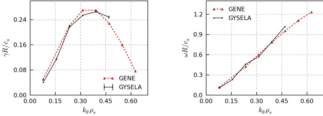
Figure 8: Benchmark between GYSELA and GENE codes for the Cyclone base Case for 6 different  $k_{\theta}\rho_s$  values: (Left) Linear growth rate (plotted with the error bar defined in Table 10), (Right) Linear frequency.
