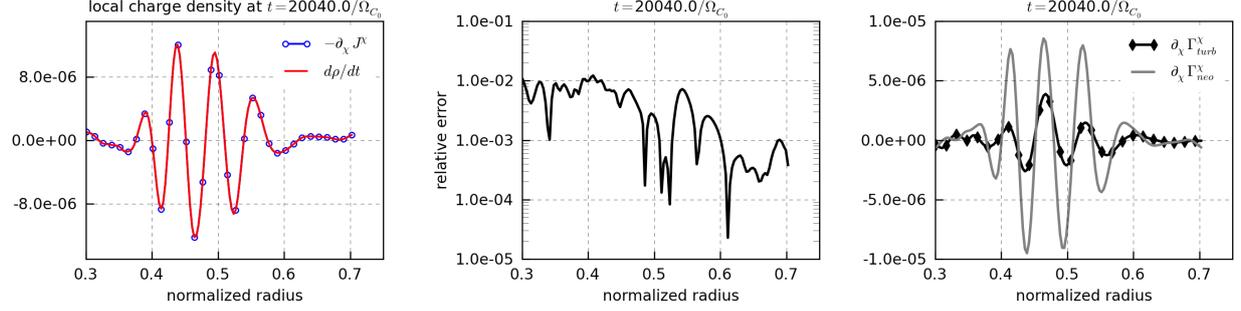
Figure 11: Numerical test of the charge density conservation for simulation defined in Table 11. All the quantities are flux-surface averaged. Left: Comparison of the two terms  $-\partial_\chi J^\chi$  and  $d\rho/dt$  which must be equivalent according to equation eq.(60). Middle: Relative error (defined as the difference normalized to the quadratic mean). Right: Contribution of the neoclassical and turbulent parts.
