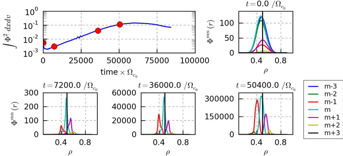
Figure 9: Radial structure of the electrostatic potential for  $(m, n) = (7, 5)$  and a bandwidth of  $m \pm 3$  modes, at different times: (i) initial time, (ii) beginning of the linear phase  $t = 7200\Omega_{C_0}^{-1}$ , (iii)  $t = 36000\Omega_{C_0}^{-1}$  and (iv) end of the linear phase  $t = 50400\Omega_{C_0}^{-1}$ .
