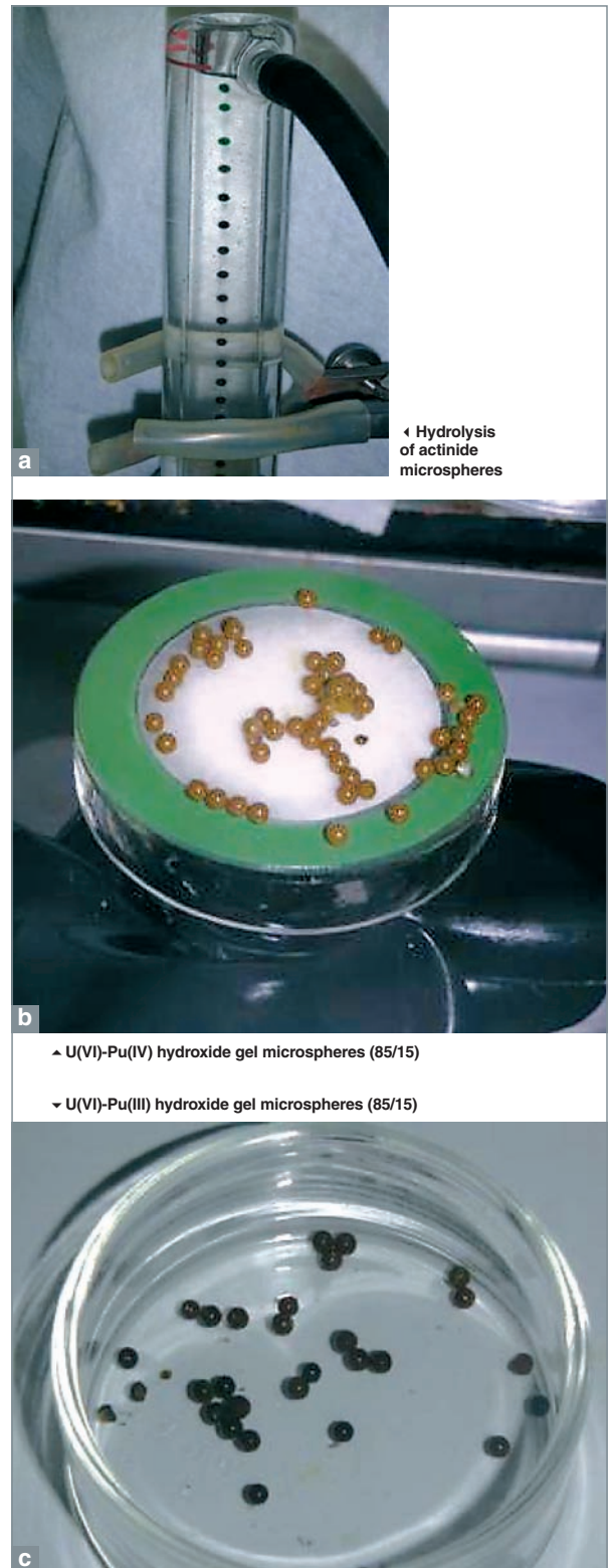
Fig. 134. Co-conversion of uranium and plutonium in a ratio of 85/15 by internal gelation.
