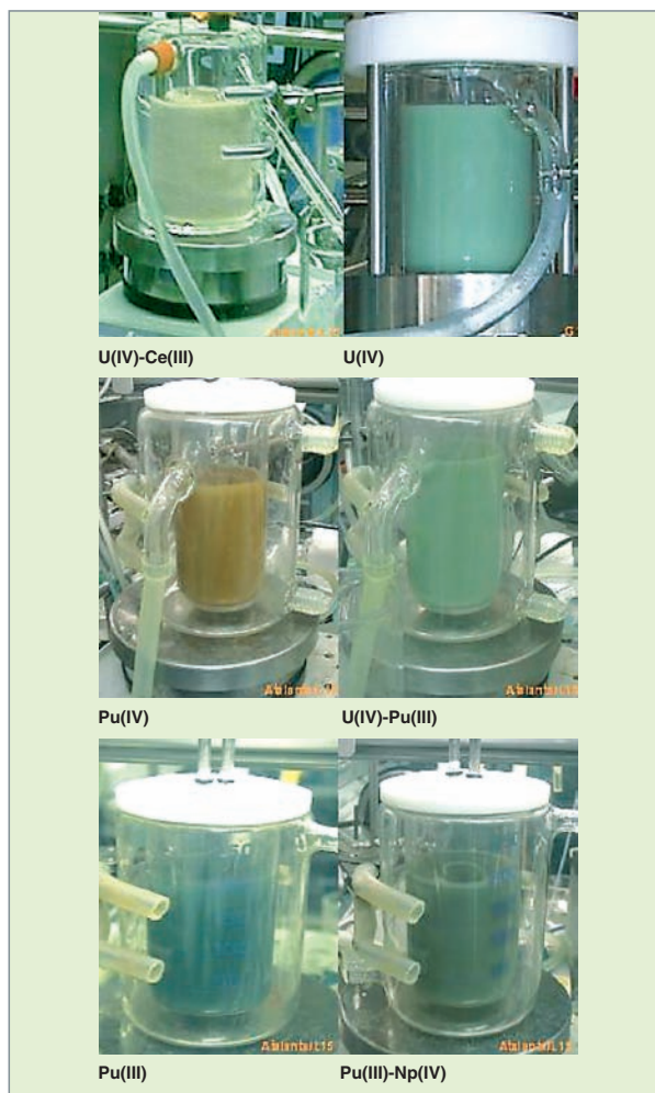
Fig. 135. Actinide co-conversion tests performed in the ATALANTE facility.
