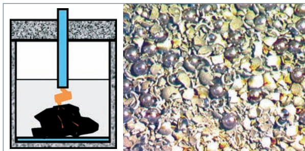
Fig. 53. Break-up of TRISO particles (ZrO 2 kernels) by pulsed current from a Marx generator (1 pulse per second - Voltage: 250 kV – Discharge time: 200 nS – Peak current: 6 kA).
