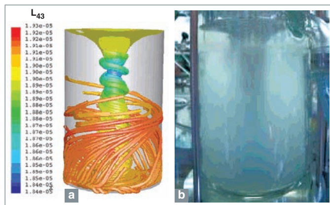
Fig. 136. Numerical simulation of the oxalic precipitation of actinides in a vortex reactor (a) and experimental setup (b) associated with granulometric monitoring of the precipitate. ( L_{43} indicates the mean volumic diameter of the uranous oxalate agglomerations.)
