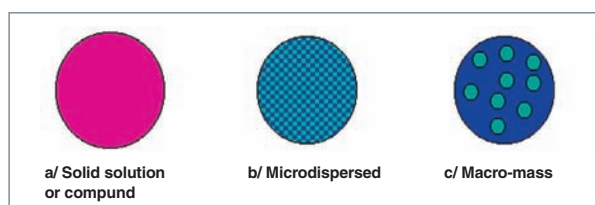
Fig. 31. The various morphologies of inert matrix fuels.
