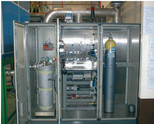
Fig. 71. Chlorinator used to synthesize zirconium tetrachloride (Zr precursor in the vapor phase ZrC deposition method) from Zr powder attacked with HCl.
