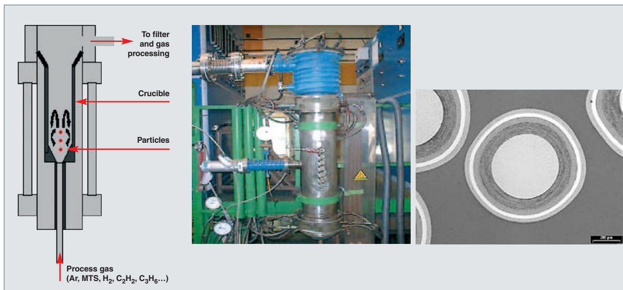
Fig. 34. The operating principle of the CVD coating process, the CEA furnace, and initial results for the coated particles.
