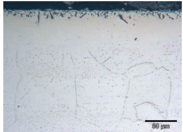
Fig. 65. Cross-sectional view of Inconel 617 (Ni <3Fe 22Cr 12Co 9Mo) after 813 hours of exposure at 950 °C to helium containing 200 vppm H_2 , 50 vppm ^{16}CO and 20 vppm CH_4 . A chromium oxide surface layer containing Ti and internal intergranular oxidation of the aluminum (initial content: 1.26%) can be observed. A carbide-free area subjacent to the surface is also observed, as well as inter and intragranular carbides closer to the core.
