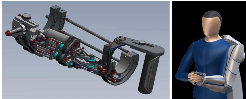
Fig 8. Right, Forearm - wrist 3 axis structure actuated by 3 SCS ; Left, Integration in ABLE 7D
