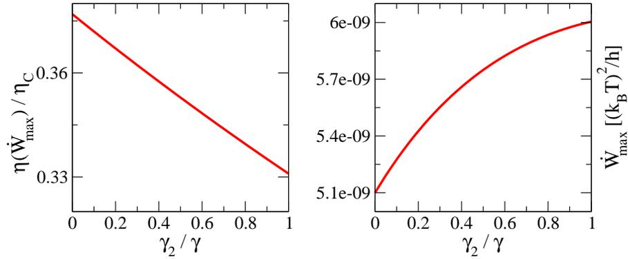
**Figure 5.** (Color online) Left panel: Efficiency at maximum power  $\eta(\dot{W}_{\max})$ , normalized over the Carnot limit, as a function of the coupling to the reservoir 2. Right panel: Maximum output power  $\dot{W}_{\max}$  extracted from the system, as a function of the coupling to the reservoir 2. Parameters:  $\gamma = 0.1 k_B T$ ,  $E_d - \mu = 2.0 k_B T$ ,  $\Delta T_1 = 10^{-3} T$ , and  $\Delta T_2 = 0$ .
