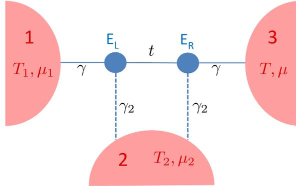
**Figure 8.** (Color online) Sketch of the double dot model used in the numerical simulations: two quantum dots with a single energy level are connected in series to three fermionic reservoirs 1, 2 and 3. The chemical potential and temperature of reservoir 3 are assumed as the reference values  $\mu$  and  $T$ . A two-terminal configuration is obtained in the case in which the coupling to reservoir 2 (equal for both the dots) vanishes ( $\gamma_2 = 0$ ).
