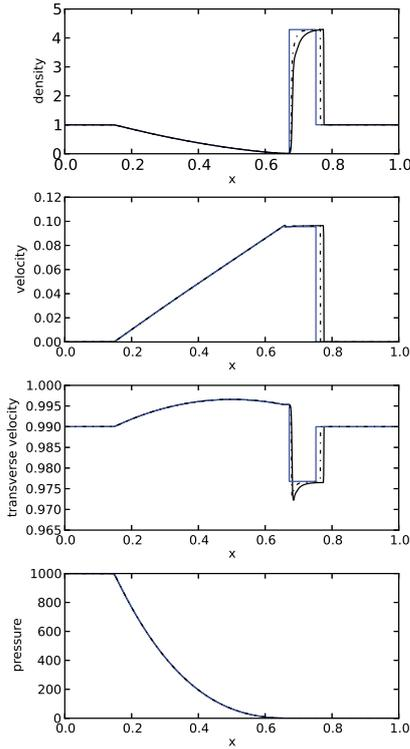
**Fig. B.2.** Inclined shock test: density, velocity, pressure and Lorentz factor along the shock normal. The thick solid lines give the 2D results, the dot-dashed lines the 1D results from a simulation with the same resolution, and the blue lines give the analytic solution. The resolution is lower than for the 1D test in Sect. B.1.
