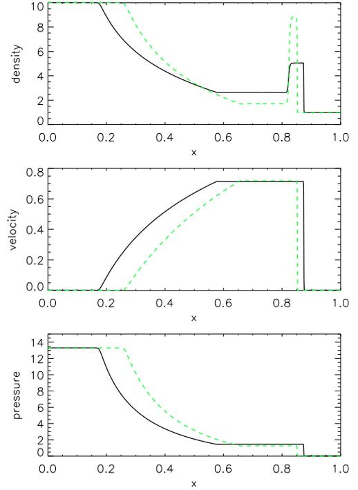
**Fig. 2.** Density, velocity, and pressure in the laboratory frame at  $t = 0.45$  for tests with different adiabatic indices. The black solid line shows  $\gamma = 5/3$ , the dashed green line shows  $\gamma = 4/3$ , the resolution is  $n_x = 256$ .
