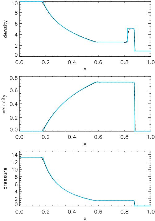
**Fig. 1.** Density, velocity, and pressure in the laboratory frame at  $t = 0.45$ . The thin solid line shows the PLM method, the dashed line the MUSCL method, which gives very similar results. The analytic solution (Giacomazzo & Rezzolla 2006) is given in blue. The resolution is  $n_x = 256$ .
