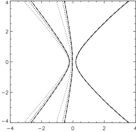
**Fig. 4.** Position of both shocks and the contact discontinuity for  $\eta_{\text{rel}} = 1$ ,  $\beta_p = 0.99$  for increasing resolution  $l_{\text{max}} = 10$  (thin dotted line), 11 (thick dotted line), 12 (dashed line), 13 (solid line). The last two resolutions give the same result.
