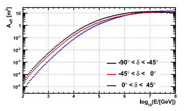
**Fig. 1.** Time-averaged muon-neutrino effective area of the ANTARES neutrino telescope as a function of energy for different declination bands  $\delta$  for the considered data-taking period. Typical quality cuts as derived in this analysis ( $\Lambda > -5.35$ ,  $\beta < 1^{\circ}$ ) are applied.
