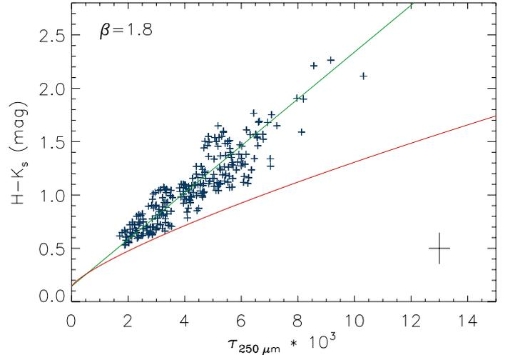
**Fig. 7.**  $H - K_s$  colours of the background stars as a function  $\tau_{250\ \mu\text{m}}$  from *Herschel* assuming a dust emissivity index of  $\beta = 1.8$ . A linear fit to the data points is shown with a green line. The red curve shows the relationship implied by the dependence of  $\sigma_{\text{FIR}}^{\text{H}}$  on  $N_{\text{H}}$  found in Orion A by [Roy et al. \(2013\)](#). The mean error of the data points is indicated with a cross in the bottom right.
