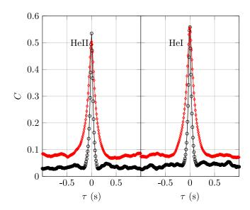
FIG. 3. Cross-correlation coefficient of the hot wire signal and of a total head pressure tube situated 4 mm apart (black ∘ 1.72 m/s and red ♦ 0.86 m/s). Measurements are performed at 45  $D_n$  from the nozzle.
