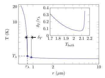
FIG. 4. Typical radial temperature profile around the wire, computed for  $T_{bath} = 1.91$  K. Inset: Thermal boundary layer in He II  $\delta_T$  normalized by  $r_{\lambda}$ , the radius of He I region.
