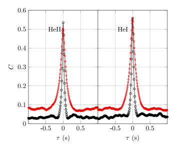
FIG. 3. Cross-correlation coefficient of the hot wire signal and of a total head pressure tube situated 4 mm apart (black  $\circ$  1.72 m/s and red  $\diamond$  0.86 m/s). Measurements are performed at 45  $D_n$  from the nozzle.
