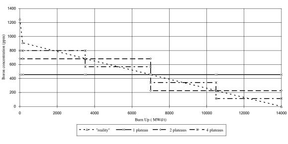
Boron history diagram with the APOLLO 1 calculation; Evolution of the concentration during an irradiation cycle.
