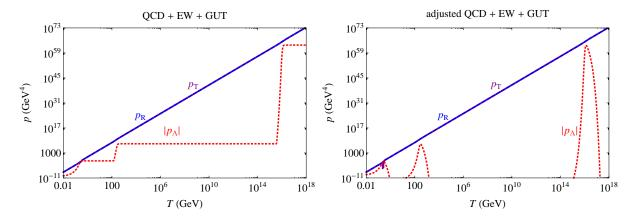
Figure 1: Sketch of the evolution of vacuum energy (dotted-red) and the total pressure (solid-purple) dominated by radiation (dashed-blue) during the expansion of the Universe. Left: standard model evolution where the vacuum energy jumps at every PT (the ones pictured here correspond to the GUT, EW and QCD PTs). Right: the evolution assuming some form of adjustment mechanism for vacuum energy.
