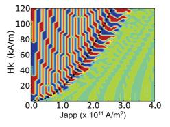
FIG. 6. (Color online) From macrospin simulations, the average in-plane component  $m_x$  of the magnetization in permanent regime vs applied current density and anisotropy field. Dark blue and red colors correspond to the equilibrium states  $\langle m_x \rangle = \pm 1$ , respectively. Light green color corresponds to  $\langle m_x \rangle = 0$ , the out-of-plane precessional steady state. The analytical critical current is represented by the black dashed line.
