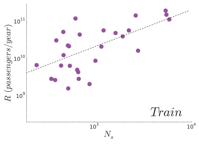
**Figure 5. (Train) Ridership and number of stations.** The total yearly ridership R of the railway networks as a function of the number of stations. A linear fit on the 47 data points gives  $R \sim 7.010^8 N_s$  ( $R^2 = 0.86$ ) doi:10.1371/journal.pone.0102007.q005
