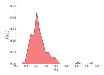
Figure 2. (Subway) Relation between the length and the number of stations. (Left) Length of 138 subway networks in the world as a function of the number of stations. A linear fit gives  $L \sim 1.13 \, N_S \, (R^2 = 0.93)$  (Right) Empirical distribution of the inter-station length. The average interstation distance is found to be  $\overline{\ell_1} \approx 1.2 \, \mathrm{km}$  and the relative standard deviation is approximately 440 m. doi:10.1371/journal.pone.0102007.q002
