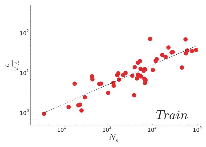
Figure 4. (Train) Total length and number of stations. Total length of the national railway network L rescaled by the typical size of the country  $\sqrt{A}$  as a function of the number of stations  $N_s$ . The dashed line shows the best power-law fit on the 50 data points with an exponent  $0.50\pm0.08$  ( $R^2=0.87$ ). doi:10.1371/journal.pone.0102007.g004
