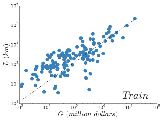
Figure 6. (Train) Total length of the network and wealth. Total length of the railway network L as a function of the country GDP G. The dashed line shows the linear fit on the 138 data points which gives  $\epsilon_L/\alpha \approx 10^4 \, \mathrm{dollars.km^{-1}} \, (R^2 = 0.91)$ . doi:10.1371/journal.pone.0102007.g006
