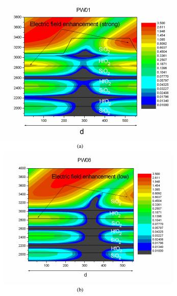
Fig. 7. Reconstruction of  $E^2$  in the top area of gratings PW01 (a) and PW08 (b)
