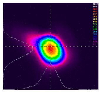
Fig. 3. Spatial profile of the focused laser used for testing. Diameter of 200 µm at 1/e<sup>2</sup>
