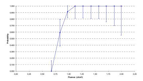
Fig. 4. Example of damage probability on a 1740 l/mm gold grating. Testing is done at an incidence of 72.5° in TM polarization. The damage threshold i.e. maximal value at which damage probability is null is 0.67 J/cm<sup>2</sup>
