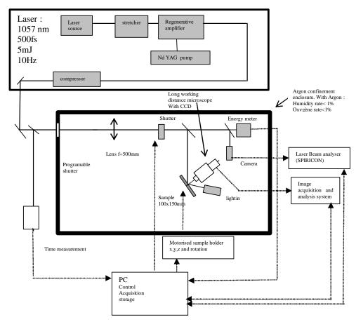
Fig. 2. Experimental setup for laser damage testing
