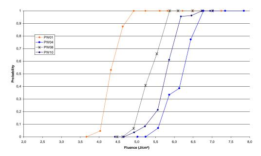
Fig. 8. Damage performance at 1.053 μm, 77.2°, TE polarization, 500 fs of 4 MLD samples
