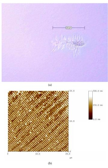
Fig. 11. Damage on sample PW01. (a) A periodic pattern perpendicular to the gratings lines is lightly visible on the periphery of the damage. (b) an AFM observation of the periodic ripple.
