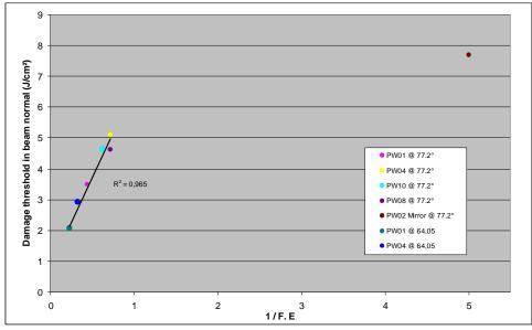
Fig. 10. Damage performance at  $1.053~\mu m$ ,  $77.2^{\circ}$  or  $64.05^{\circ}$  of incidence, TE polarization, 500 fs versus  $1/E^2$  maximum on four different MLD samples and a mirror (PW02).
