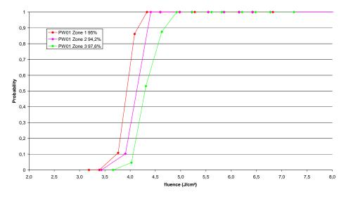
Fig. 9. Damage performance at 1.053  $\mu$ m, 77.2°, TE polarization, 500 fs on different zone of PW01 sample with corresponding measured diffraction efficiency
